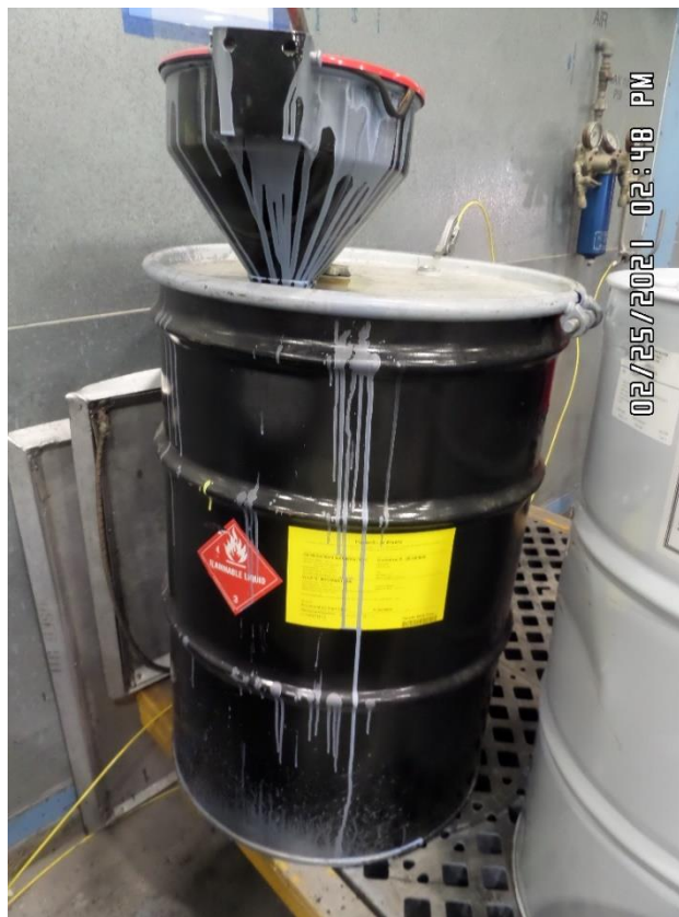
Figure 1 - 55-gallon SAA container storing paint waste
