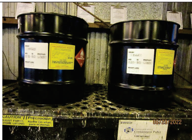
Photograph #2 - Building (b) (3) (A) - two closed 20-gallon satellite containers of waste paint related materials (D001, D005, D007, and D008) in location APS-WAP-5.
