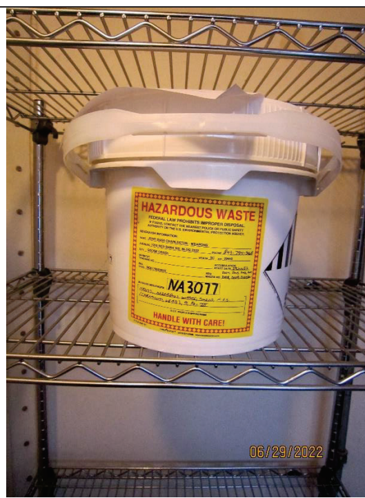
Photograph #16 - Permitted Storage Building (b) (3) (A) – One 0.6-gallon container accumulating chromium and lead waste (D007 and D008).
