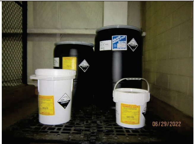
Photograph #12 – Permitted Storage Building (b) (3) (A) - three corrosive hazardous waste (D002) containers ranging from 2-gallon to 35-gallon stored in the caustic cell.
