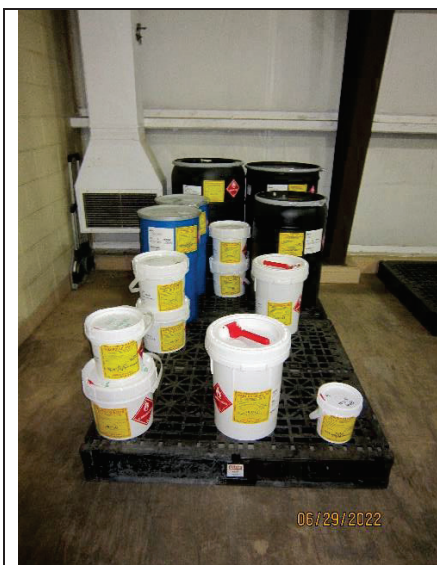
Photograph #13 – Permitted Storage Building (b) (3) (A) - fourteen hazardous waste containers ranging from 0.6-gallons to 55-gallons storing spent solvents, gasoline, fuel filters, compressed gas, and paint.
