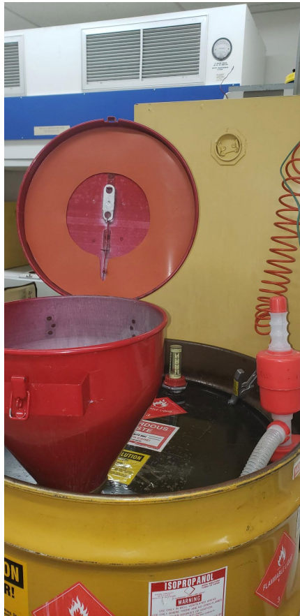
(Figure 1: Shows a funnel with a gasket on top of a 55-gallon drum.)
