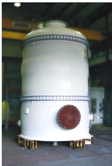
Fig. 3: Contact surfaces coated with fluoropolymers
