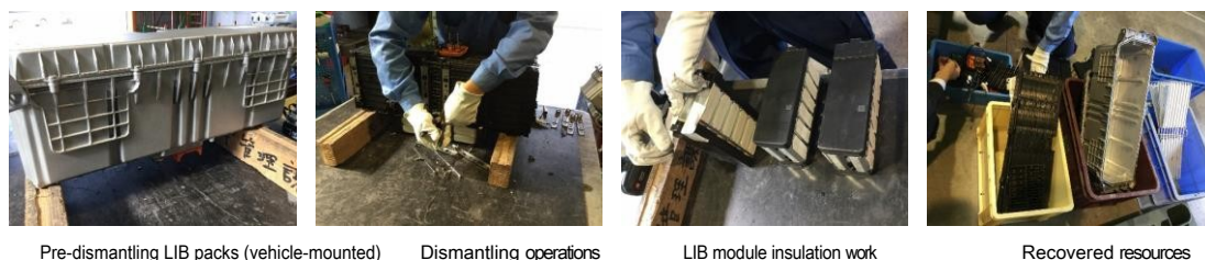
Figure 1-5. Disassembly and manual disassembly of used LIB packs in this demonstration project
