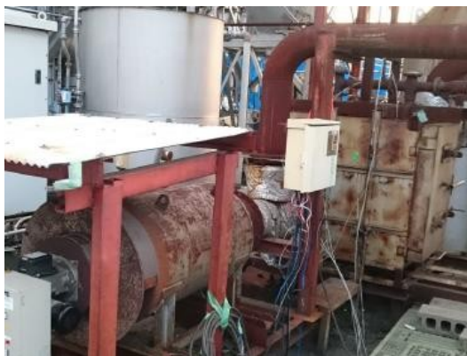
Figure 1-7. Roasting furnace in this demonstration project (Hiroshima Gas Techno Service) (Remark: the size of the furnace interior is 560 mm (W) x 1000 mm (D) x 900 mm (H))
