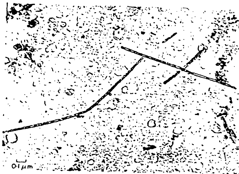
FIG. 3. Single fibrils filtered from London air. The fibril dia. is about 0.04 \mu\text{m} , typical of chrysotile. The fine structure shows changes similar to those observed when chrysotile is heated.
