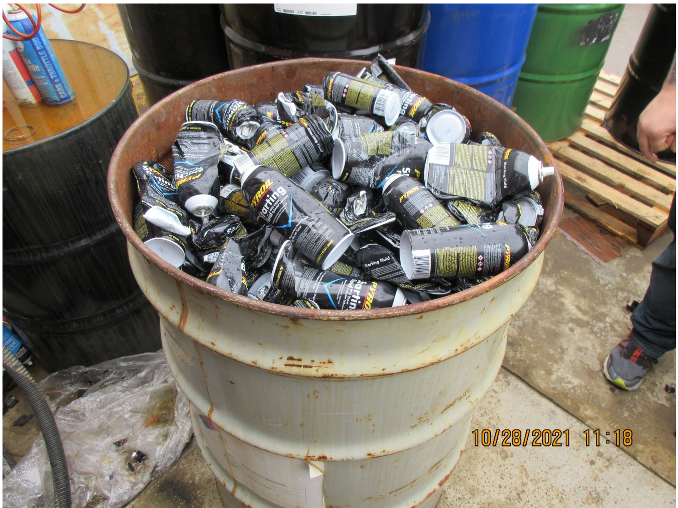
Photo 12 – Containers with solvents to be recovered and blended back into products
