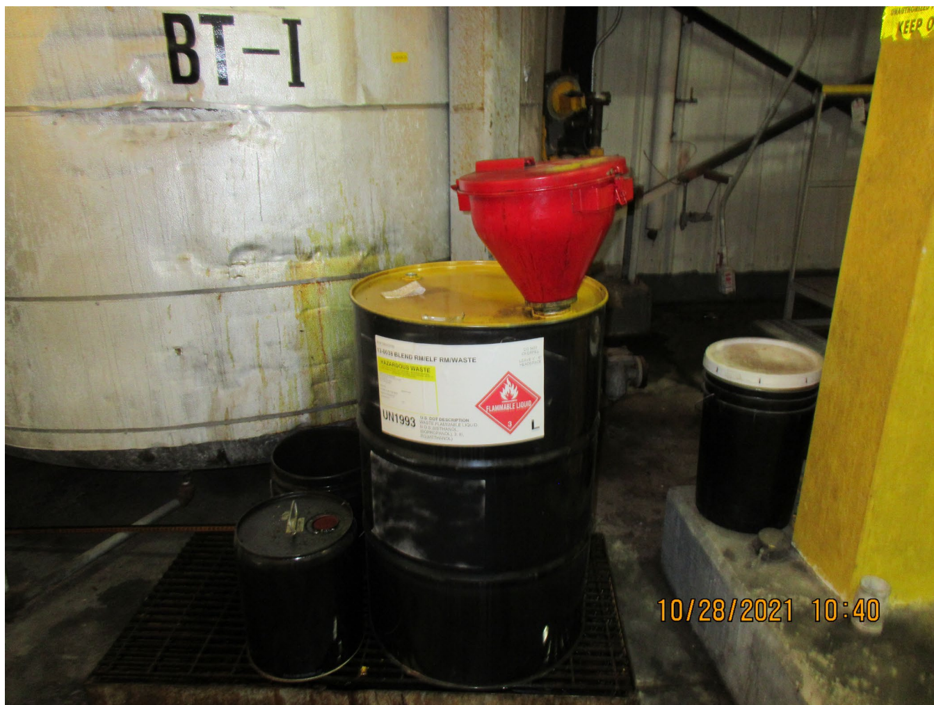
Photo 3 – 55-gallon container of hazardous waste in SAA in the Blend Room and 5-gallon container (front left) of contaminated rags.
