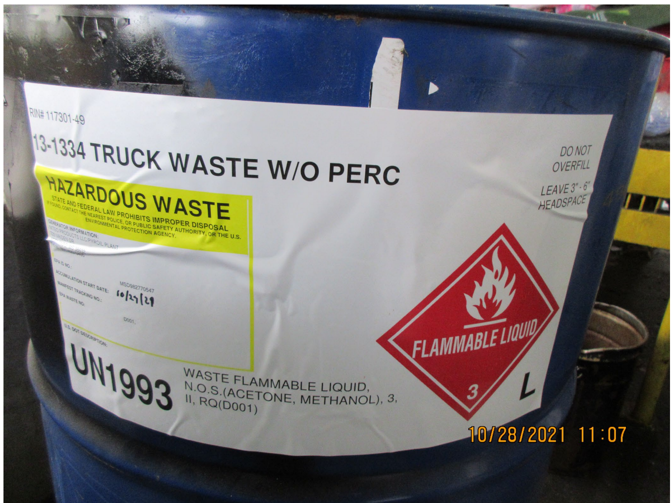
Photo 10 - Container of Hazardous Waste Liquid in SAA # 6
