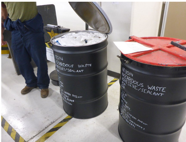
Photo 17: Two 55-gallon drums of D010 / D035 hazardous waste adhesive / sealant located at the Workcenter 51A SAA in the Air Frames Division area. The total volume of waste exceeded 55-gallons at this SAA, and the excess waste was neither marked with an accumulation start date nor removed to a CAA or the permitted storage area.
