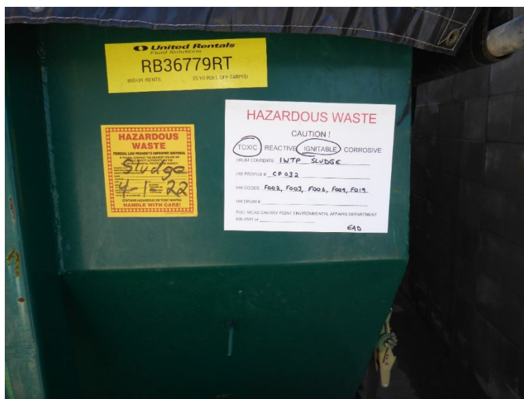
Photo 15: Indication of the hazards and accumulation start date added to one 25-yard roll-off of hazardous waste IWTP sludge.
