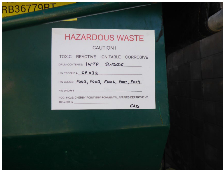
Photo 14: One 25-yard roll-off of hazardous waste IWTP sludge with no indication of hazards or accumulation start date. The SOP at the facility is to either circle the indication of hazards on the pre-printed label or to cross out those hazards that do not apply to the contents of the drum.
