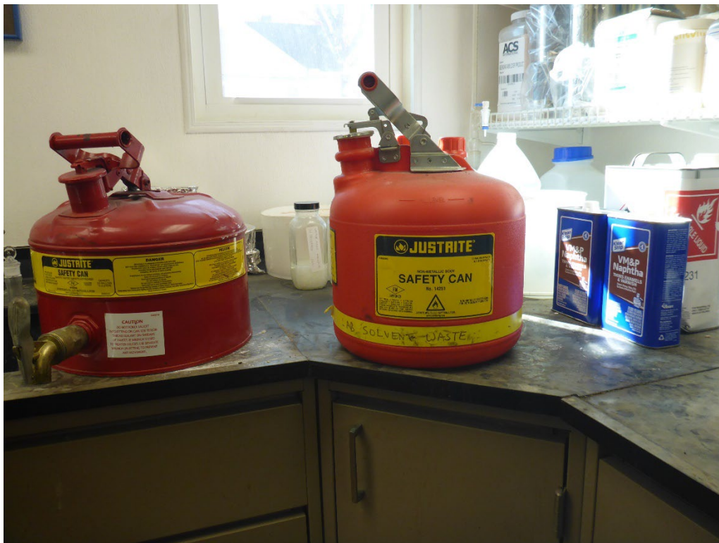
Photo 4: 2.5-gallon flammable safety can in the laboratory SAA, which was not labeled with the words “hazardous waste.”
