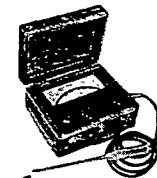
Alnor Thermo-Anemometer. For accurate measurement of low air velocity. Compact, direct-reading, battery operated, self-contained, portable. Scale 6 in. Meter ranges: 0-600 fpm and double range 0-300/100-2000 fpm. Accurate readings as low as 5 fpm. Temporary Bulletin 913-A.
