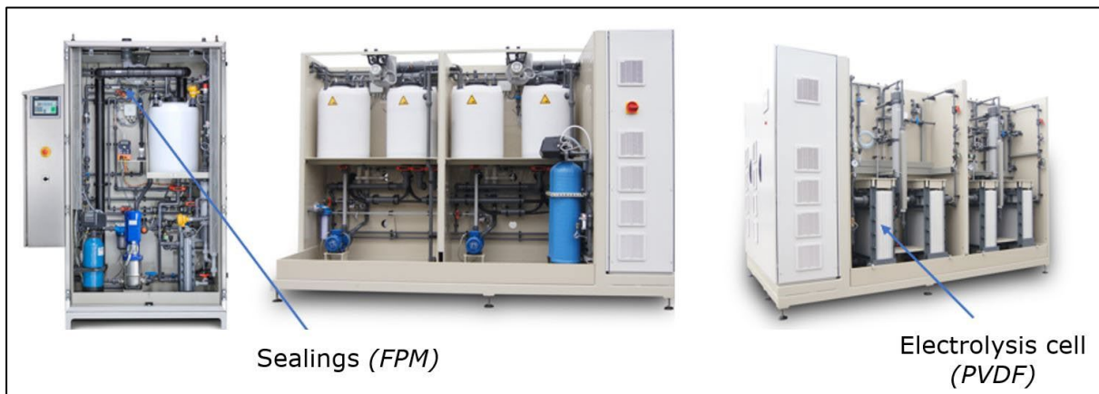
FIGURE 6: FLUOROPOLYMER-CONTAINING COMPONENTS IN AN ELECTROLYSIS WATER TREATMENT PLANT.
