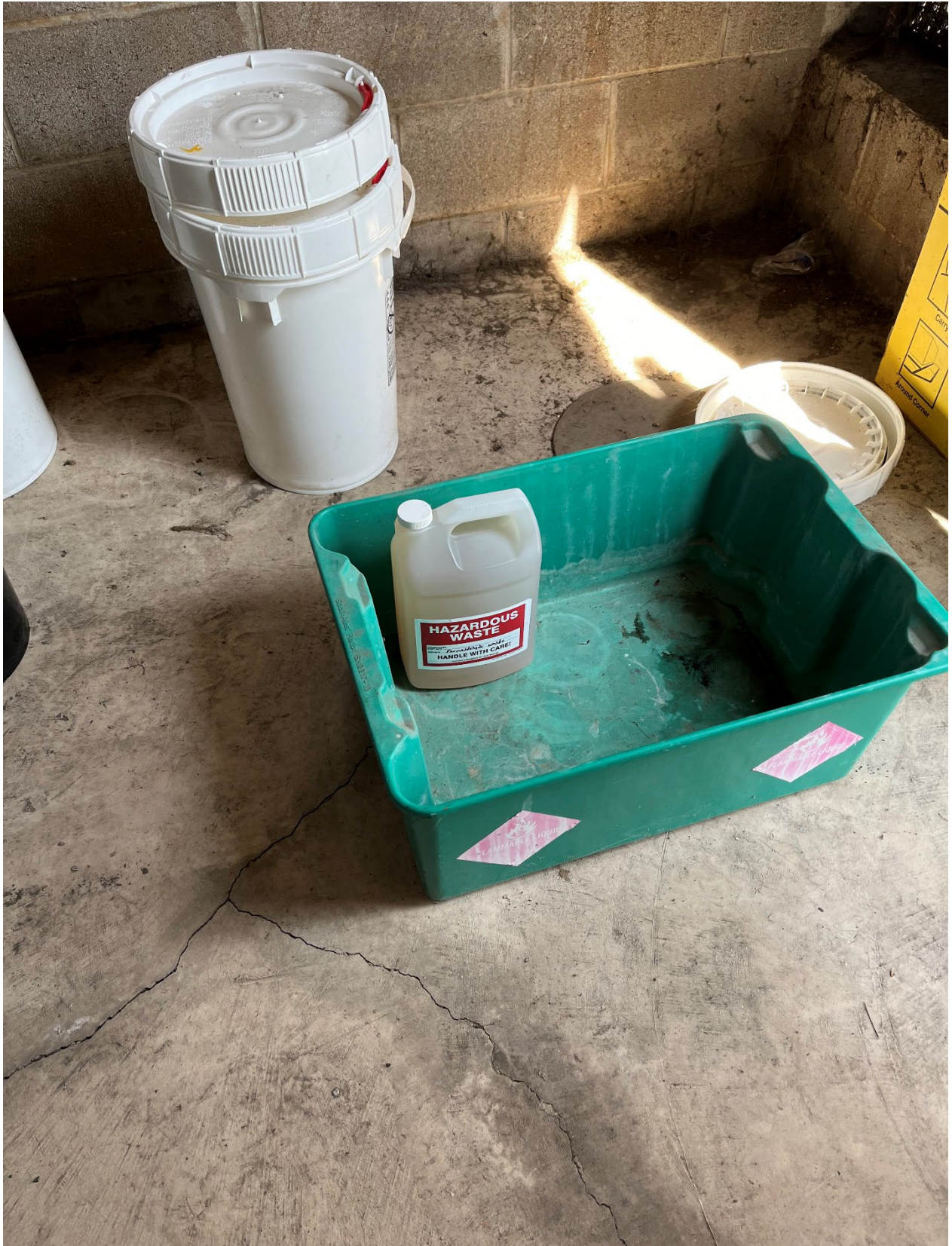
Photo #4: View of the container of formaldehyde waste with no accumulation start date.
