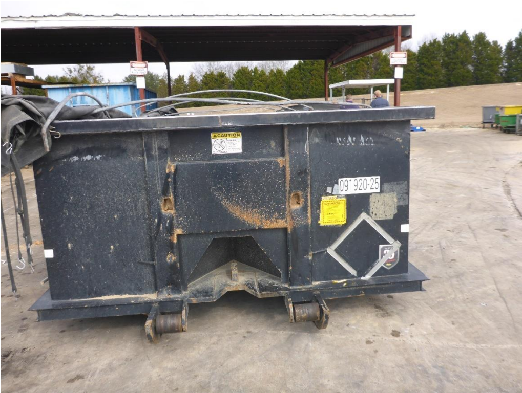
Photo 35: Roll-off container staged to receive supersacks of D008 hazardous waste baghouse dust. The container was labeled D008 hazardous waste solid (contains copper, lead and zinc) and identified with the UN3077. The container was dated 02/09/2021.
