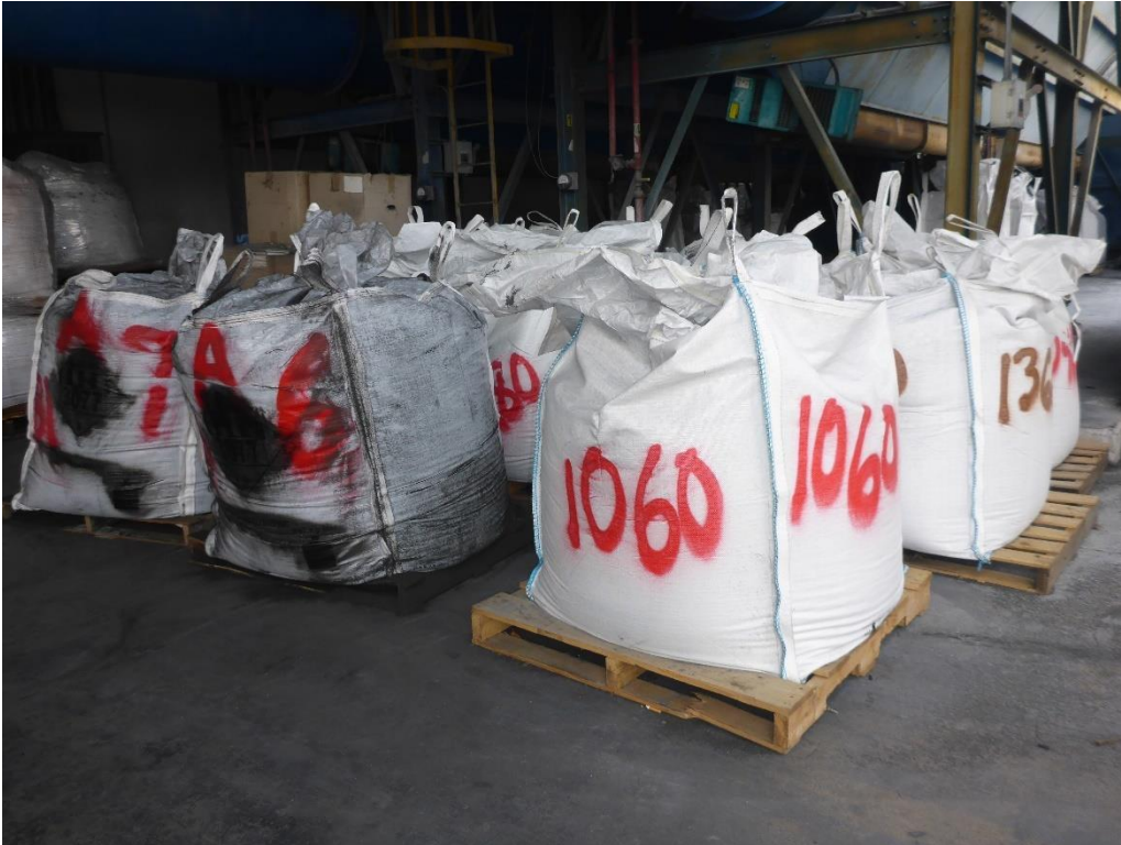
Photo 30: Supersacks observed in the Baghouse area. Bags were not labeled, but facility personnel stated they contain zinc material that will be sold for use off-site. Spray painted numbers indicate the weight of the bag.
