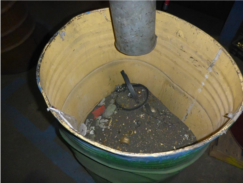
Photo 7: 55-gallon drum of used shot blast and debris generated by the Grinding Wheelabrator unit. Used shot blast and metals are reclaimed. Shot blast that is recovered in the Reclaim Room is reused on-site in the Wheelabrator; metals that are recovered in the Reclaim Room are remelted and reused in the casting process; foundry sand that is segregated in the Reclaim Room is disposed of as D008 hazardous waste. The container was open and it was not labeled.
