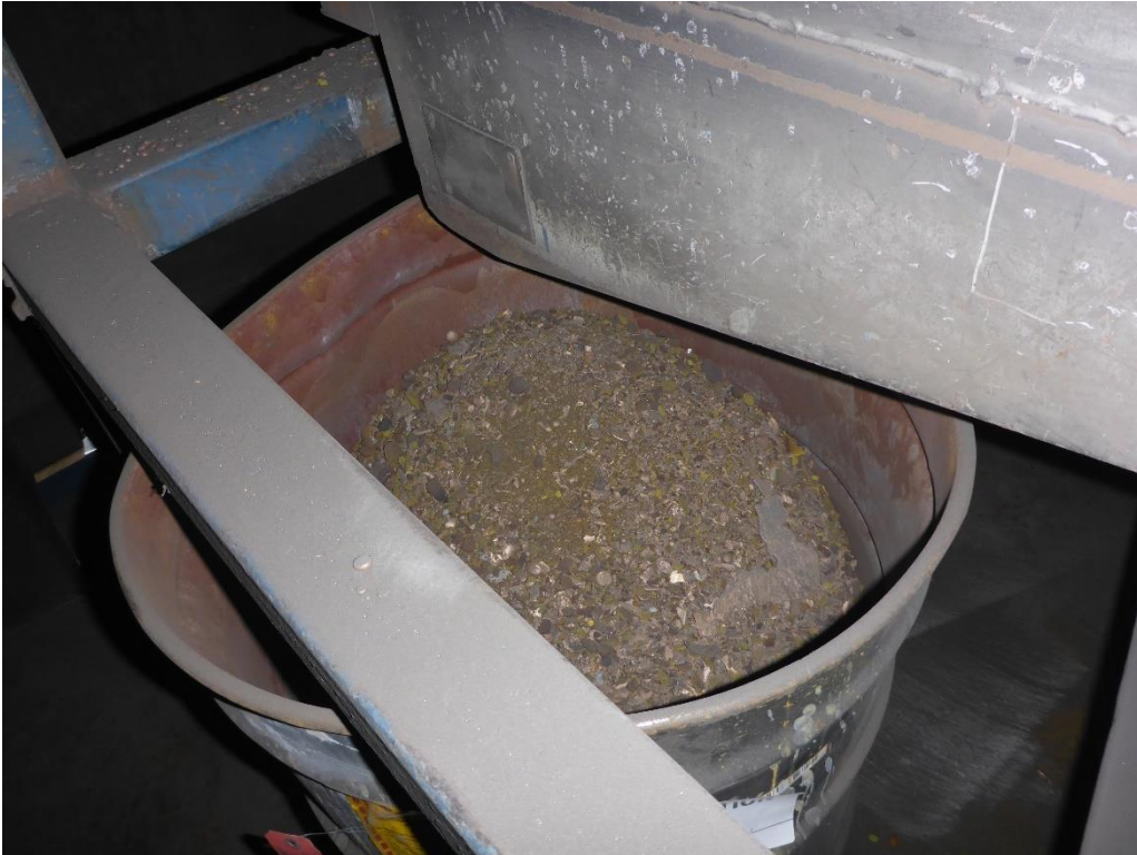
Photo 13: 55-gallon drum for accumulating separated material that has been processed in the Reclaim Room. The 55-gallon drum is labeled D008 hazardous waste 02/08/2021 and appears to contain metal shavings.
