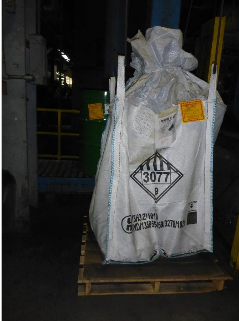
Photo 2: Supersack under one of the bleed-out chutes used to accumulate mold sand that is discharged from the storage tank so that the tank can be replenished with new sand. Supersack is labeled D008 hazardous waste solid contains copper, lead and zinc, and marked with an accumulation start date of 02/08/2020.
