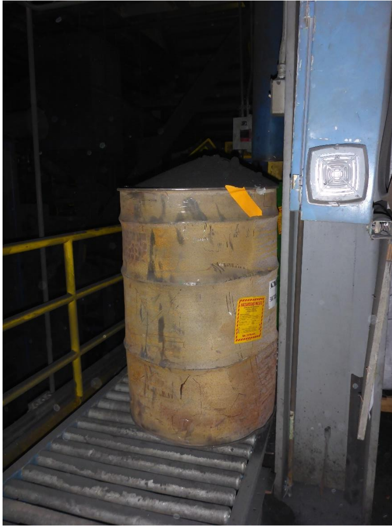
Photo 4: The third 55-gallon drum near Bleed-out area. The drum is labeled D008 hazardous waste containing copper, lead and zinc, and it is marked with an accumulation start date of 02/08/2021. The drum is overfilled, and it has no lid.
