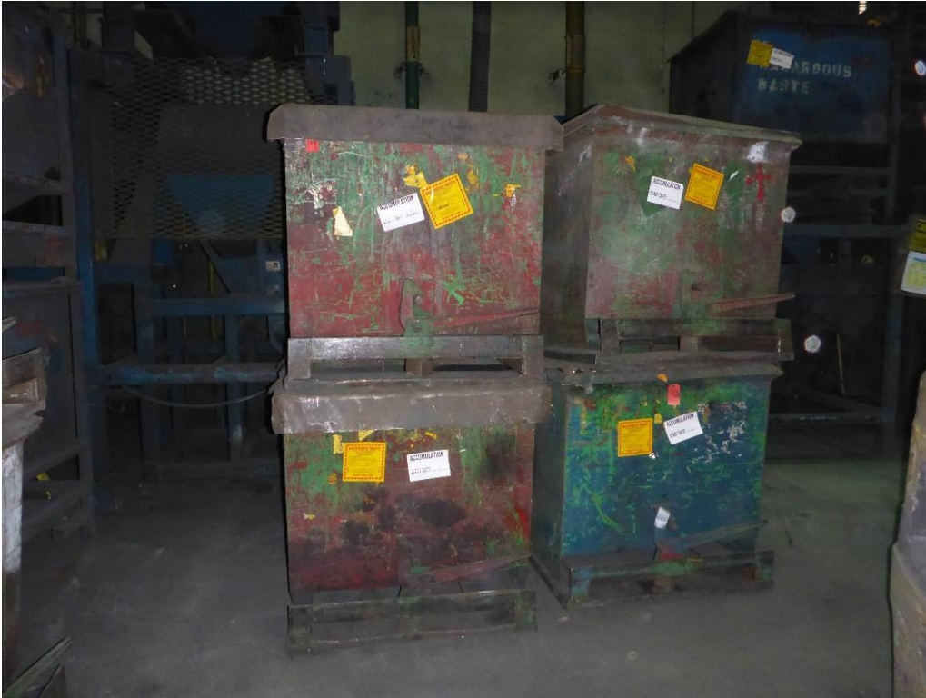
Photo 16: Metal hoppers near the door in the Reclaim Room. This area contained a total of ten metal hoppers. Eight of the hoppers were empty, and all were labeled D008 hazardous waste and marked with an accumulation start date. The oldest hopper was dated 02/01/2021. Personnel did not know if the hoppers contained material ready for reclamation or material that had already gone through the separation process.
