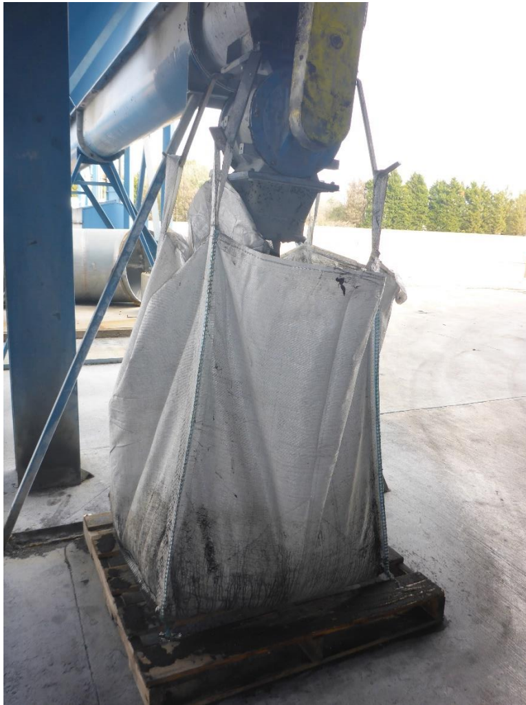
Photo 33: Supersack observed under the Travel Vent Baghouse. Bag is not closed, labeled as hazardous waste, or marked with an accumulation start date.
