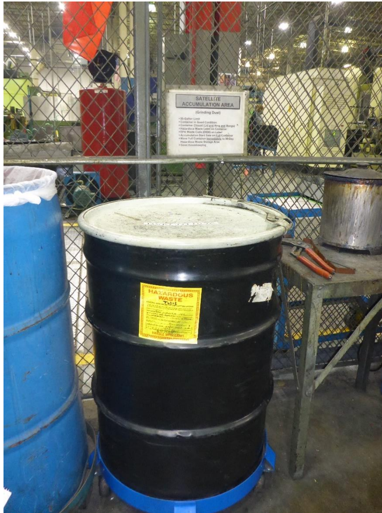
Photo 24: SAA for accumulating air filters generated in the air handling vacuum system in the Tool Crib area. The drum was labeled D006 hazardous waste solid led and identified with the word “toxic” on the hazardous waste label. Not that the D006 hazardous waste characteristic is toxic for elevated levels of cadmium, not lead.
