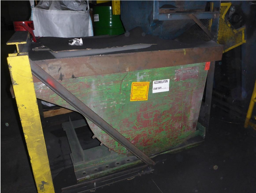
Photo 6: Green hopper containing excess used mold sand coming off the conveyor belt. Facility personnel stated that this material is dumped back into the system for reuse on-site. The container was labeled D008 hazardous waste containing copper, lead and zinc, and it was marked with an accumulation start date of 02/08/2021.
