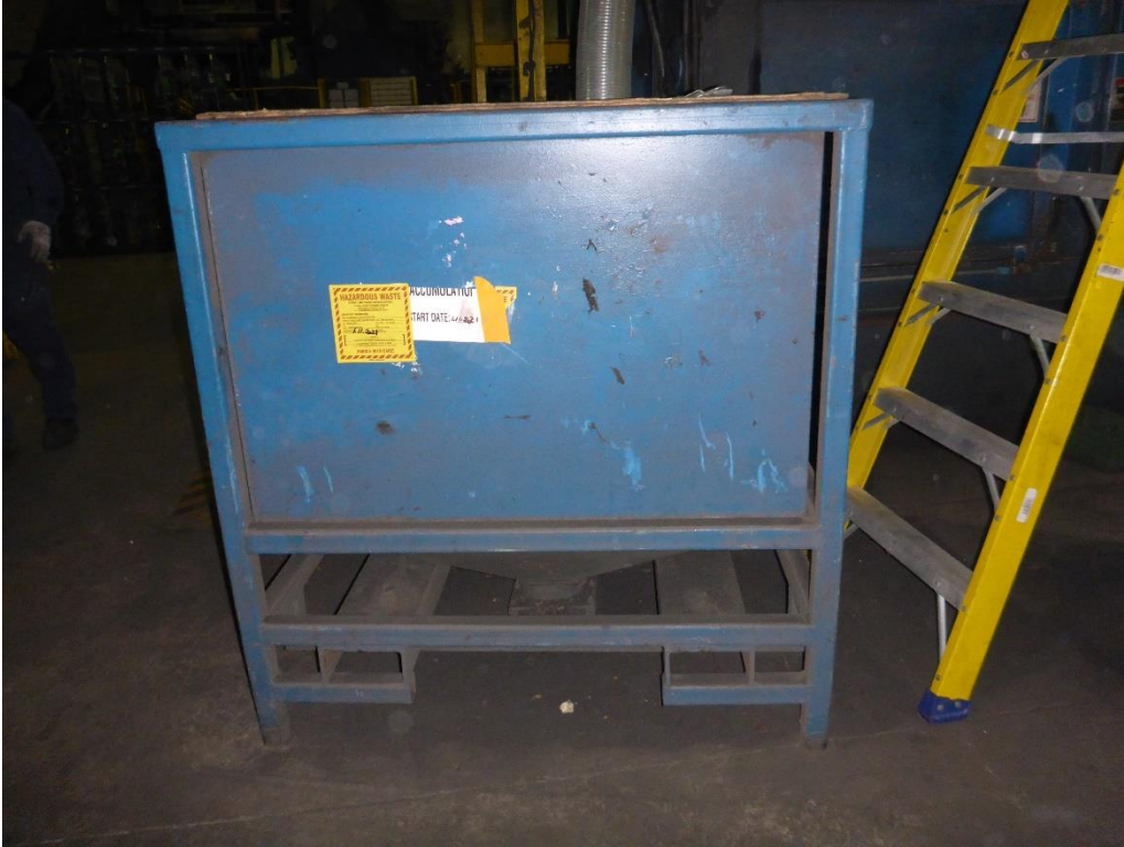
Photo 1: Blue box for accumulating core mold pieces that will be sent for brass recovery on-site. Box is labeled hazardous waste solid D008 contains copper, lead and zinc and marked with an accumulation start date of 01/11/2021.
