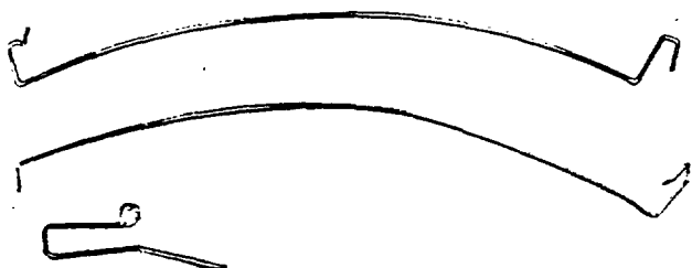
5. Only first course of lath requires crimping of wire. Other courses are rapidly applied by looping field clips over channel and inserting hook into the eye of the preceding clip.
