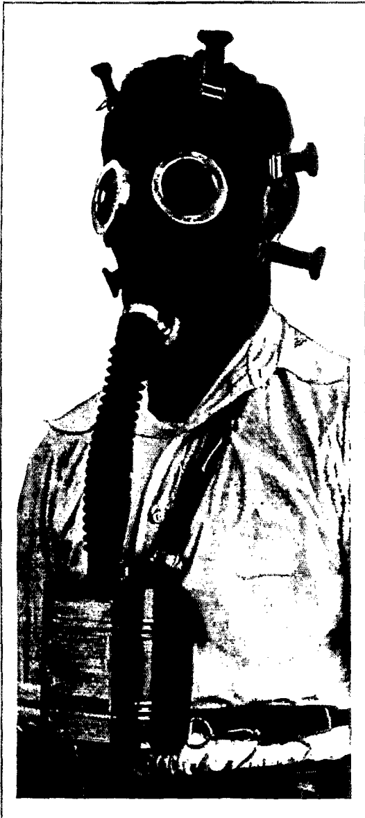
M-I Type Canister Mask with 650 cc Canister
