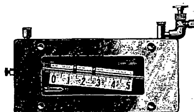
SINGLE-TUBE INCLINED: This gage is for small boilers and furnaces, and for power boilers with operating draft not over the scale range of ½ inch. It is equipped with seal for 400 feet chimney height, natural draft.
