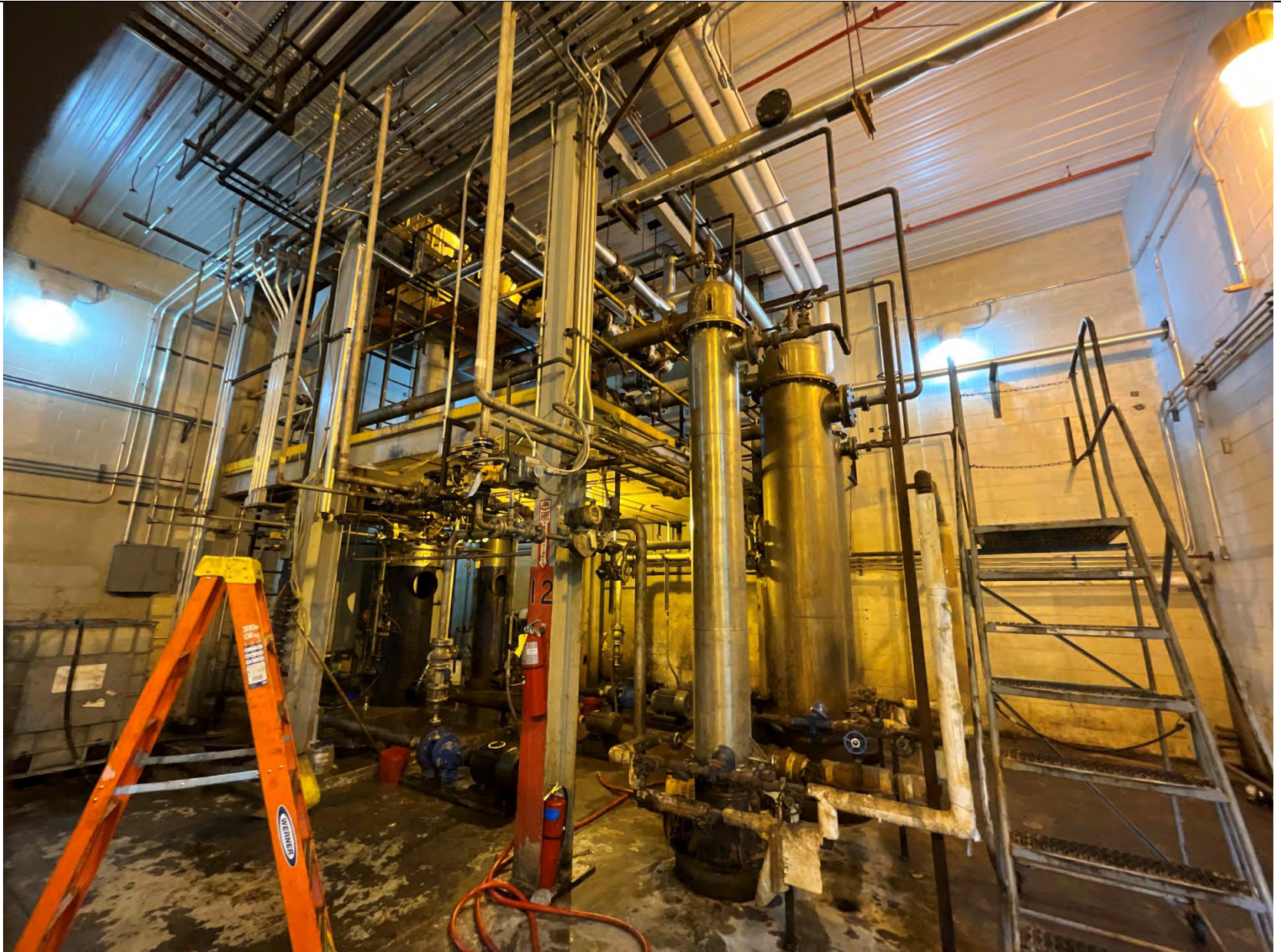
The distillation units where methanol is extracted from the glycerin.
