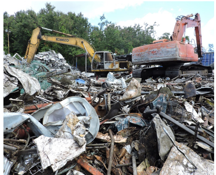
Picture 24 - DCN RECYCLING, CORP. - As observed by the EPA Inspector at the Ferrous Metal Collection Area, scrap metals are first segregated by metal properties, crushed with the excavator to reduce metals size, and then immediately sent to the cargo trucks.
