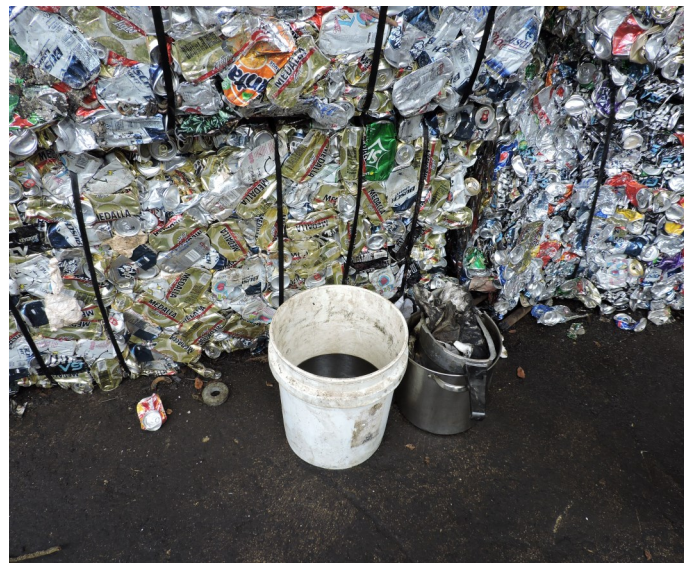
Picture 22 - DCN RECYCLING, CORP. - As observed at the Machine Shop Area, there was one (1) 5-gallon plastic container open and with used oil not properly labeled with the words, "Used Oil."
