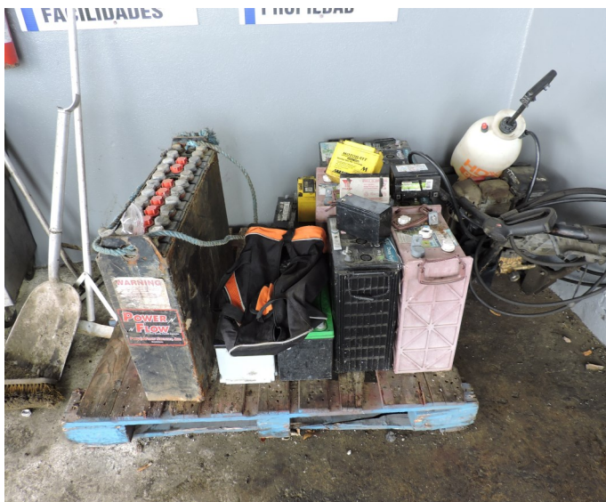
Picture 11—DCN RECYCLING, CORP. - Approximately twenty-five (25) discarded auto batteries placed on a wood pallet without any means of containment measures or labels. According to Ms. Cordero a battery carrier would be contacted to recycle the auto batteries at the Entrance Gate and Weighing Scale Area.
