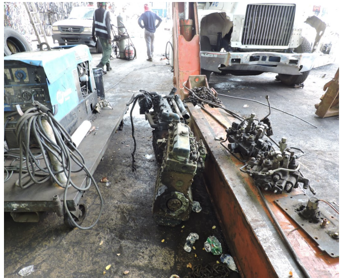
Picture 10 - DCN RECYCLING, CORP. - At the Entrance Gate and Weighing Scale Area, dismantled motor engines with no control or prevention of releases of used oil or stormwater runoff contaminated with transmission fluids, gasoline, diesel, and other motor oil fluids.
