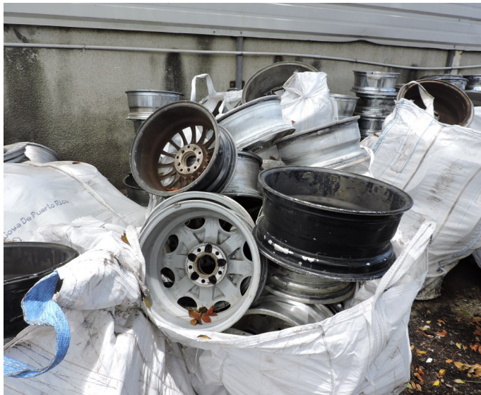
Picture 31—DCN RECYCLING, CORP. - At the Alloy Wheel Collection Area, all alloy wheels are received, collected and packed in 1-cy white cloth bags. It was observed the most alloy wheel rims contained lead weights were not properly removed before packaging.
