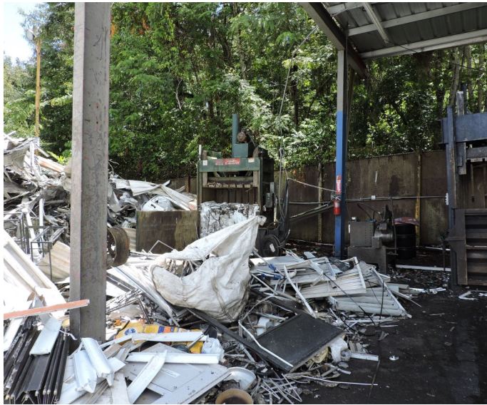
Picture 13- DCN RECYCLING, CORP. - EPA Inspector observed aluminum scrap metals are first segregated by metal properties (i.e., aluminum cans), crushed with compacting machines to reduce metals size, and then immediately transferred to 1-cy white cloth bags.
