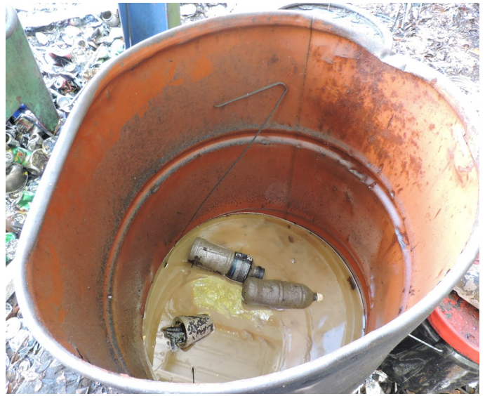
Picture 14 - DCN RECYCLING, CORP. - As observed, at the Entrance Gate and Weighing Scale Area there two (2) 55-gallon steel drums open with used oil waste content not properly labelled with the words, "Used Oil," and surrounded with scrap metals heavily impacted with used oil.
