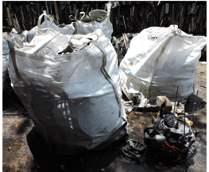
Picture 18 - DCN RECYCLING, CORP. - At the Material Processing & Storage Area there were approximately four (4) 1-cy yard “white cloth” bags with motor engine parts and other metals leaking used oils on the concrete floor without any means of control.
