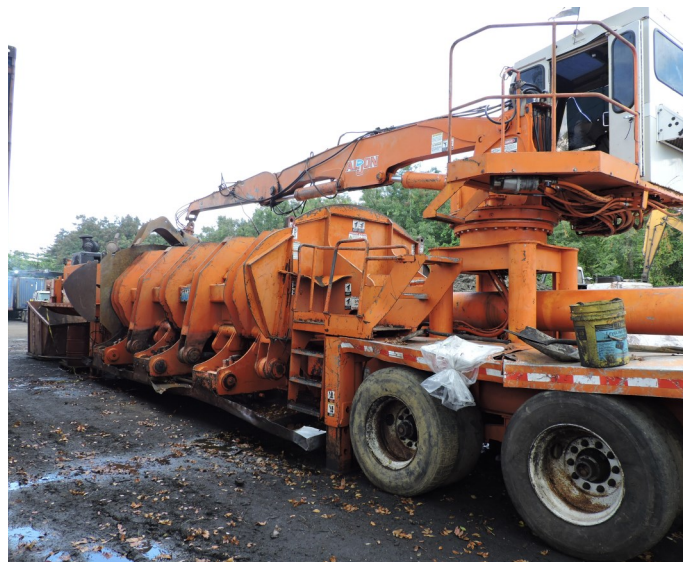
Picture 32 - DCN RECYCLING, CORP. - The EPA Inspector proceeded to inspect the Compacting Cars Area where crushing and bailing of junked cars is performed. using an ALJON 580 CL machine (i.e., crusher, bailer) at the site.
