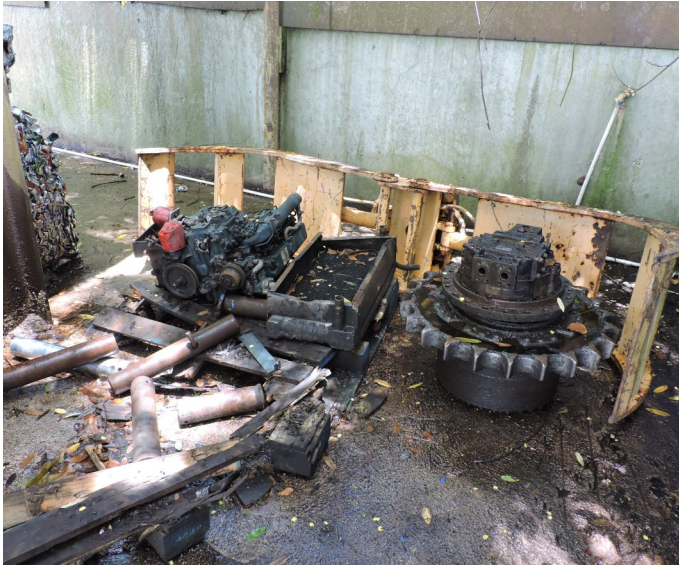
Picture 21- DCN RECYCLING, CORP. - As observed at the Machine Shop Area, dismantled motor engines with no control or prevention of releases of used oil or stormwater run-off contaminated with transmission fluids, gasoline, diesel, and other motor oil fluids.
