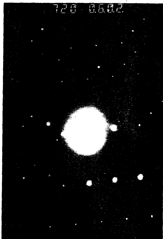
FIGURE 6. Selected-area electron diffraction pattern obtained from a single fibril of presumptive tremolite asbestos fibers detected in the lung.
