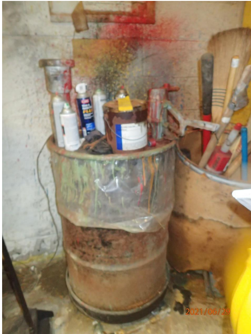
Photo 3: 55-gallon SAA drum equipped with an aerosol can puncturing device on top, open, and no label.
