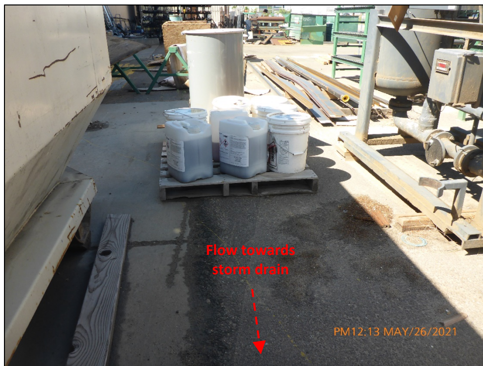
Photograph 27. View of totes of liquid glue stored outside near the trash compactor without overhead coverage or secondary containment. The totes are located upgradient of the storm drain connected to the sand/oil separator and Outfall SW1, as depicted in Photographs 4 and 5.
