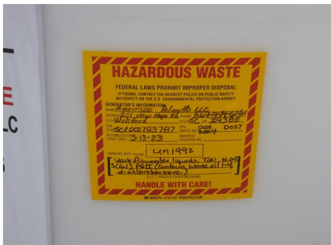
Photo 8 – Hazardous Waste Tote: Label on 300-gallon tote identifying the contents as D001, D004, D027 flammable and toxic hazardous waste, and marked with an accumulation start date of March 13, 2023.
