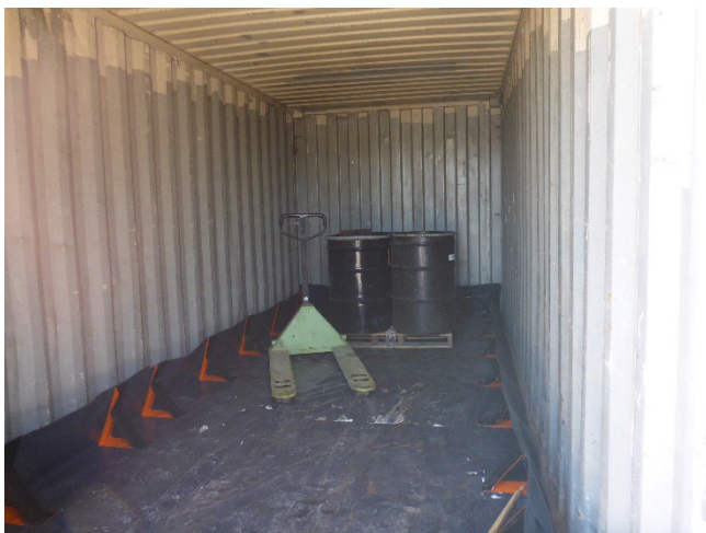
Photo 3: Four 55-gallon drums inside a trailer box car, which is the designated hazardous waste central accumulation area (CAA).
