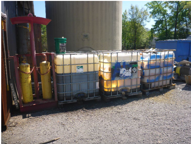
Photo 2: 275-gallon used oil tote (on the left) labeled nonhazardous waste, but not labeled with the words used oil.
