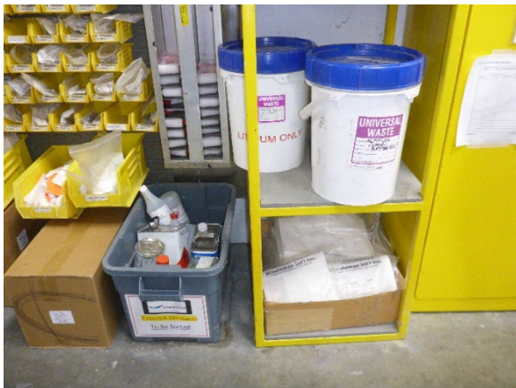
Photo 10: Two 5-gallon containers for accumulating universal waste batteries and one 10-gallon bin for accumulating empty containers and small containers of unused or expired products generated in the Composite Shop.
