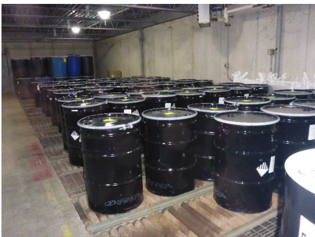
Photo 25: Approximately sixty 55-gallon containers of hazardous waste in the third storage section in the main CAA. Each container was labeled D001, D006, D007, D035, F003, F005 hazardous waste flammable solids (acetone, xylene), and marked with an accumulation start date. The oldest container was dated February 26, 2024. Although the containers were each identified with a DOT class 9 hazard sticker, none were marked with an indication that the contents are toxic.
