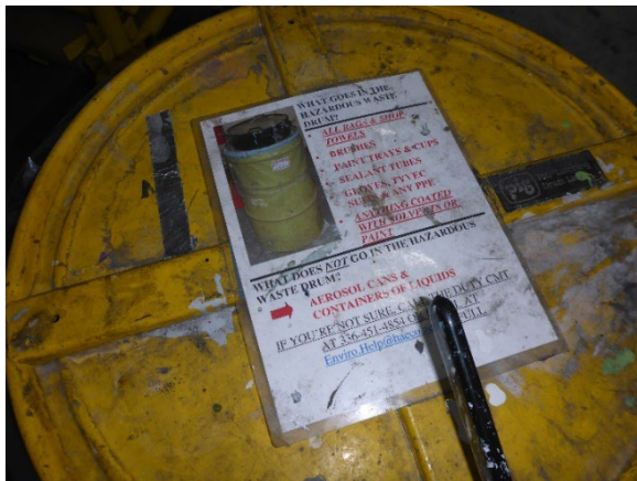
Photo 2: Notice on top of the container shown in Photo 1 which instructs personnel on what materials may and may not be placed inside the container.
