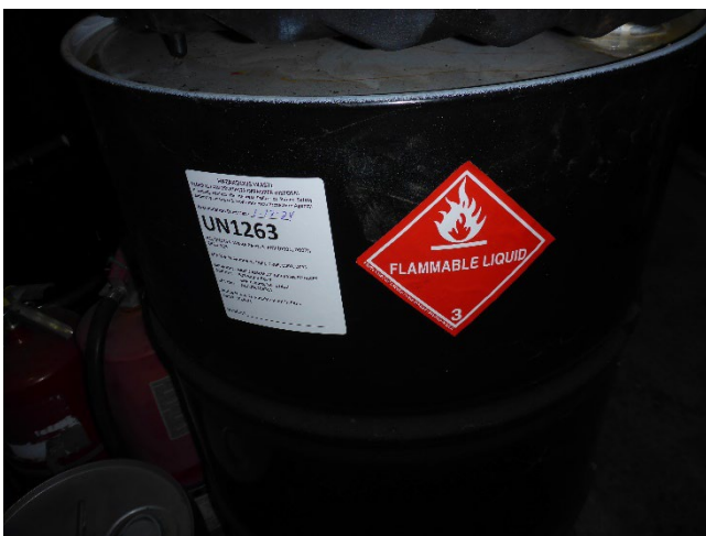
Photo 22: Label on active 55-gallon container at the start of the first of three storage sections that run length-wise through the main CAA building. Container used to consolidate waste paint thinner solvent as hazardous waste.
