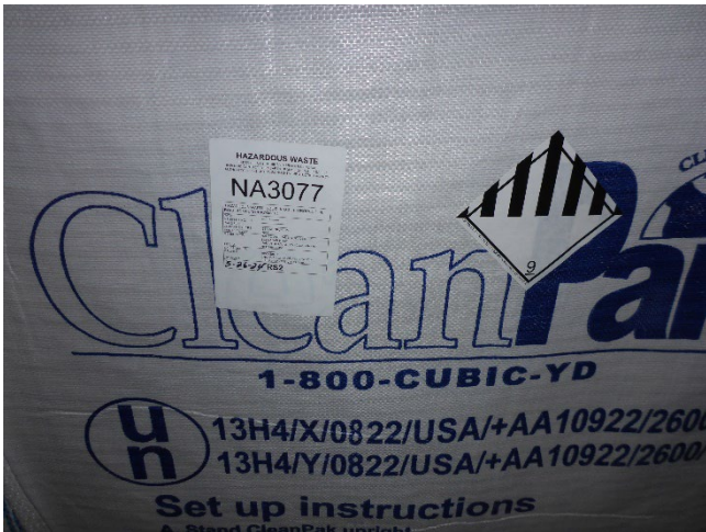
Photo 24: Supersack of hazardous waste observed in the second storage section of the main CAA. The supersack was labeled as hazardous waste solid contaminated paint filters, marked with an accumulation start date of March 26, 2024, and identified with a DOT class 9 hazard sticker. It was not marked with an indication that the contents of the container are toxic.
