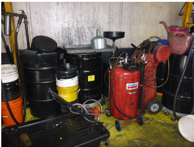
Photo 15: One 55-gallon container of used oil, one 55-gallon container of used oil filters and one 55-gallon container of used antifreeze among other equipment in the GSE Shop. Stains on the wall, containers and equipment show evidence of poor housekeeping.
