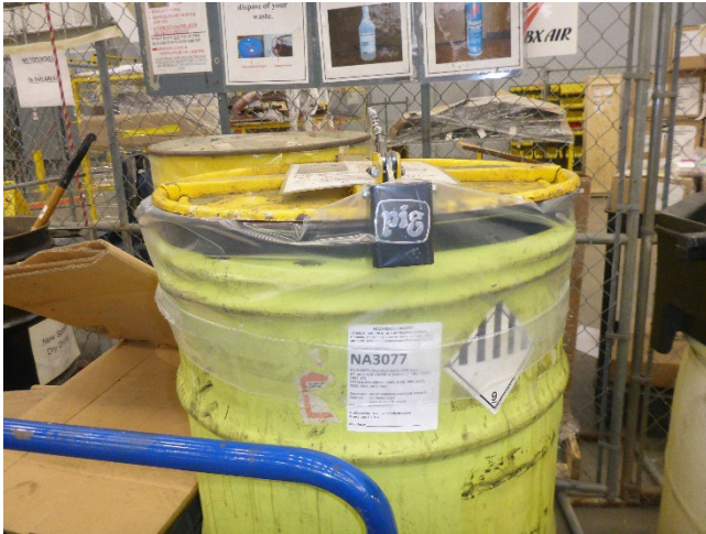
Photo 17: One 55-gallon container in a Hanger #4 mobile SAA. The container was labeled D005, D006, D007, D008, D035, F002, F003, F005 hazardous waste debris, gloves, rags, and PPE, but it was not marked with an indication of the hazards of its contents.
