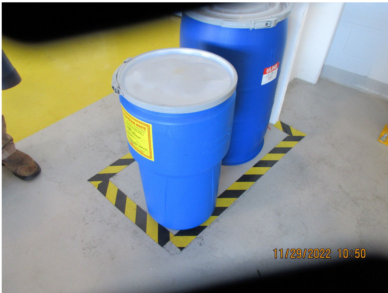
Photo 2 – Container in VMFAT – 501 Area – Building 3090 without hazard indicator
