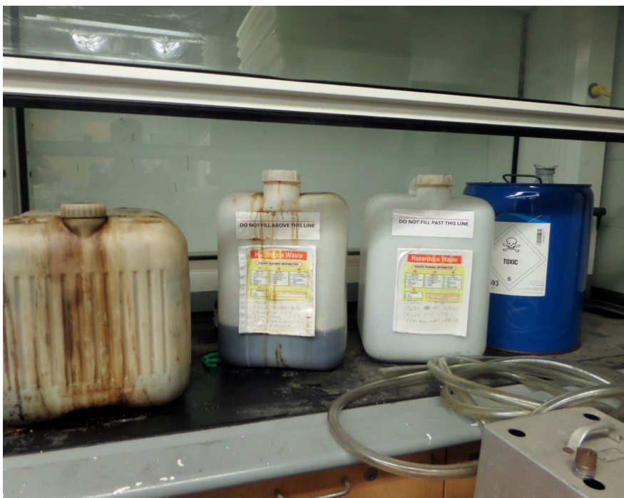
Photo-11 Chemistry Physics Building – CP34 Indication of hazards of contents not marked, Spilled Contents, Expired chemicals, Containers in bad condition
