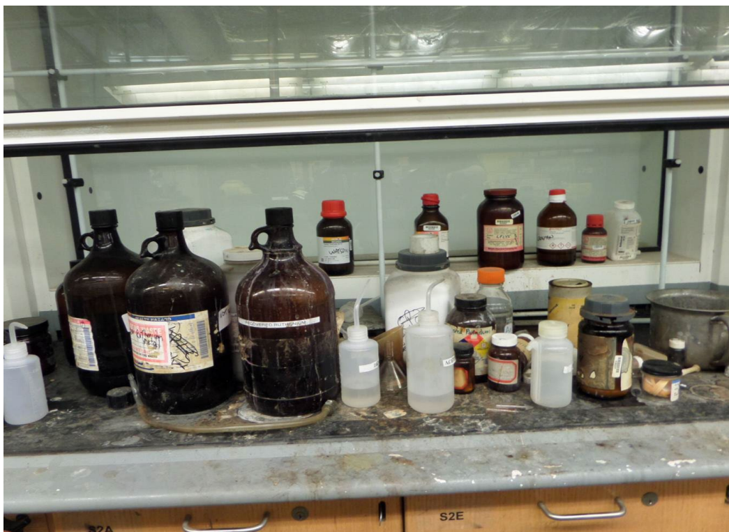
Photo-8 Chemistry Physics Building – CP34 Indication of hazards of contents not marked, Containers in bad condition Discarded and Expired Chemicals, Stains on the Countertop
