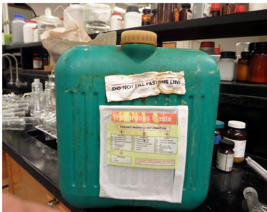
Photo-7 Chemistry Physics Building – CP8 Indication of hazards of contents not marked
