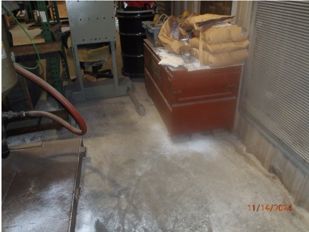
Picture 26 – Breaker Shop Zero Blast Cabinet spilled media
