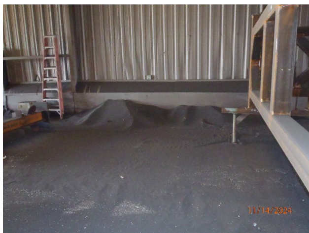
Picture 48 – Shop 2 Blaster Shop spent media from lead abatement
