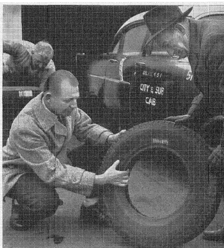
Ability of nylon tires to take punishment was verified in taxicab tests. Tire above was the champ; it lasted through 12 retreadings.
