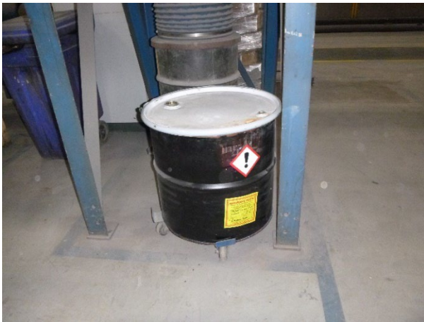
Photograph 7: Coating Booth Dust SAA.
