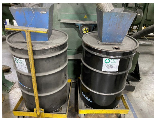
Photograph 37: Goff blaster shot for recycle.
