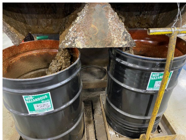
Photograph 35: Goff blaster sludge waste.
