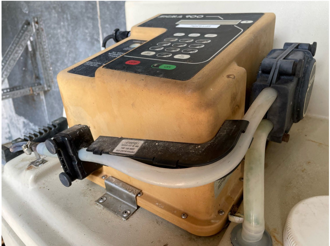
Photograph 6: Algae was observed in the silastic tubing of the composite effluent sampler.
