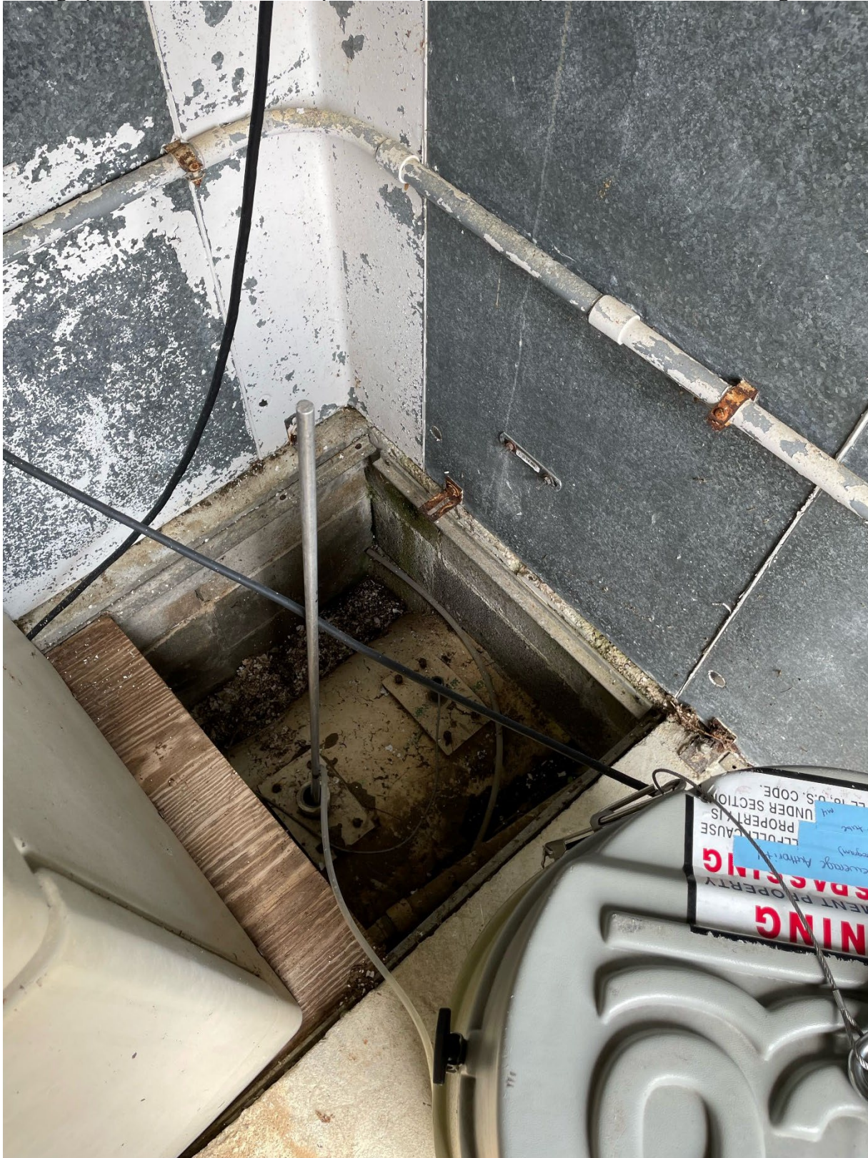
Photograph 1: EPA automatic composite sampler was setup at the effluent monitoring location
