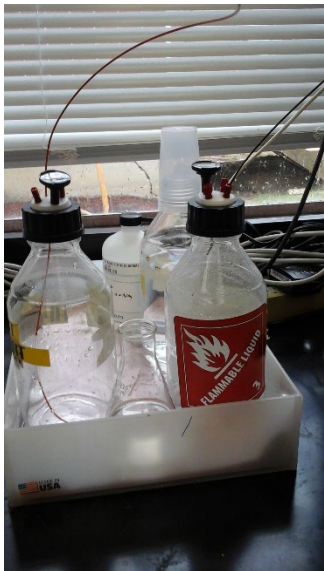
Photo 7: 1000-mL SAA container in QC Laboratory missing a hazardous waste label.
