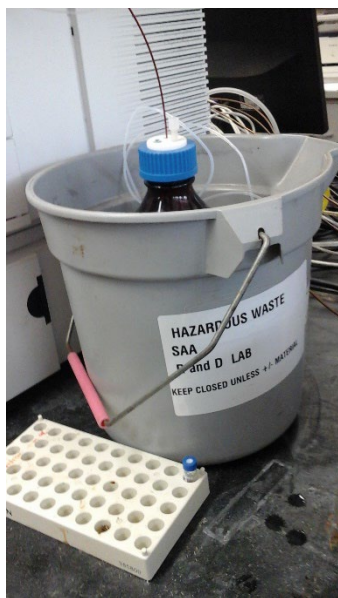
Photo 3: SAA 1800-mL container in R&D laboratory, missing an indication of the hazard of the contents.
