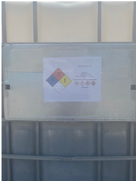
Photo 3: Used Oil label placed on oily water tote.
