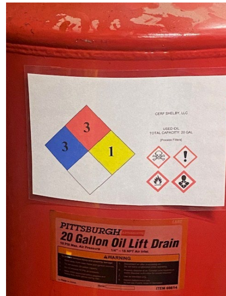
Photo 12: 20-gallon used oil container inside Maintenance Warehouse.
