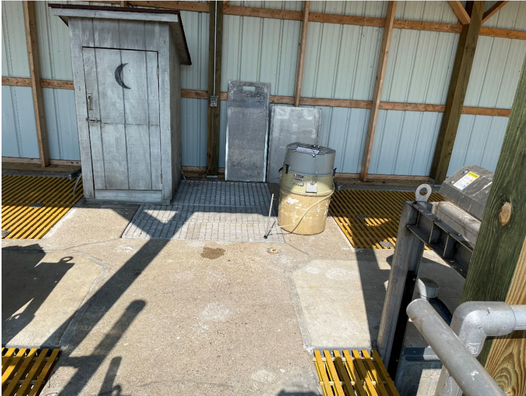
Photo #1. EPA automatic composite sampler was set-up at the effluent receiving pit.
