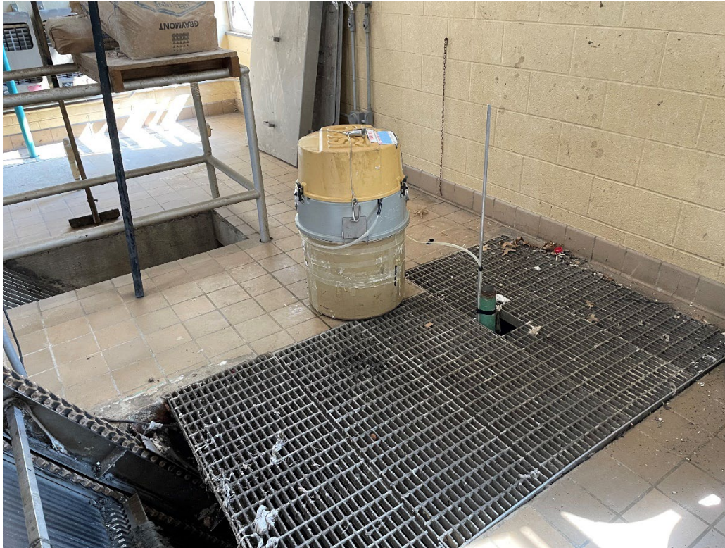
Photo #2. EPA automatic composite sampler was set-up at the influent sampling point.
