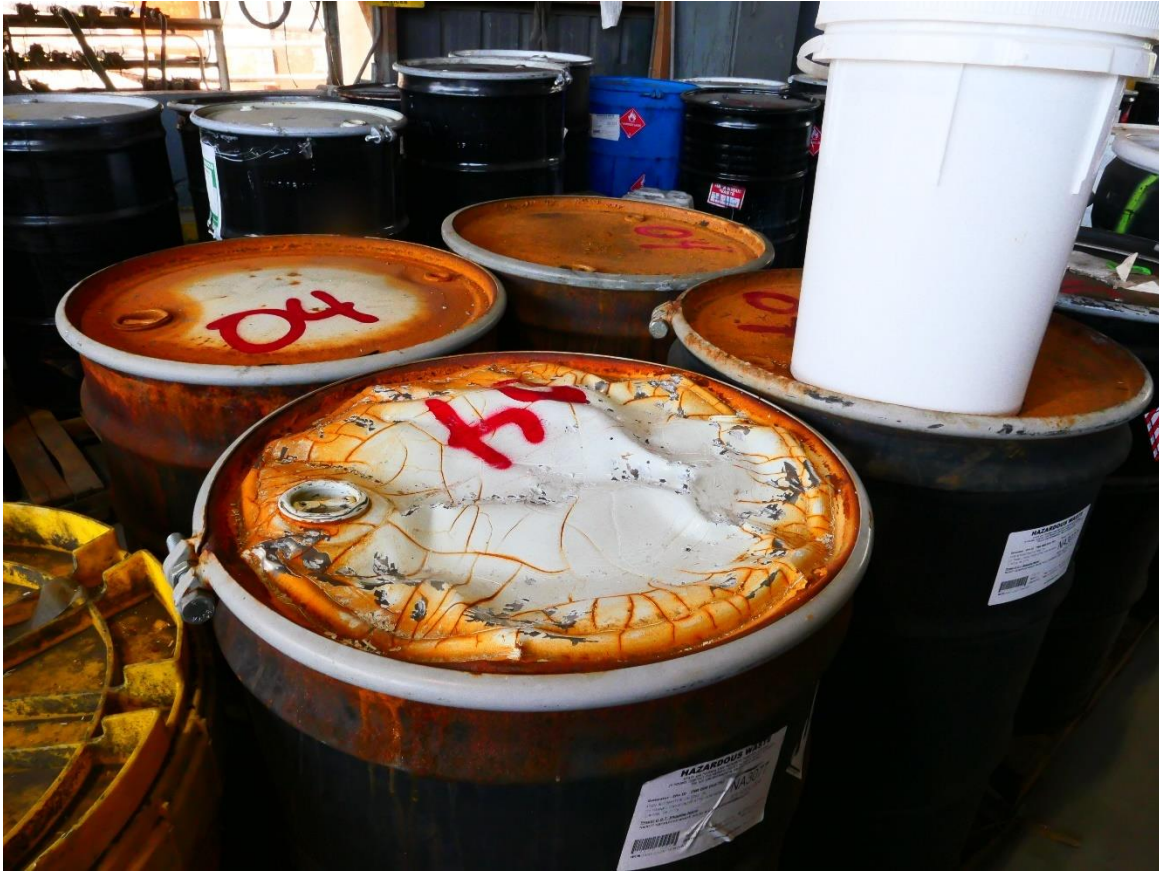
Photo 19: Rusted drums with damaged/ dented top.
