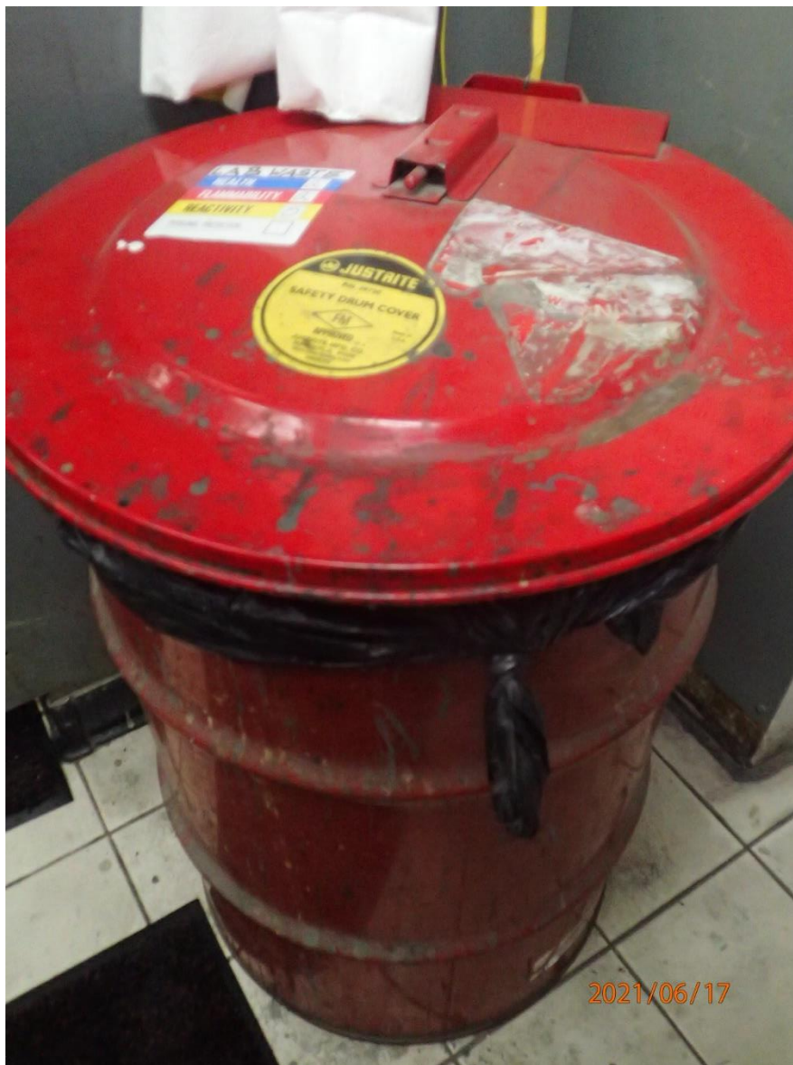
Photo 1: 55-gallon drum labeled “Lab Waste”, closed, with a hazard identification sticker marked for flammability.
