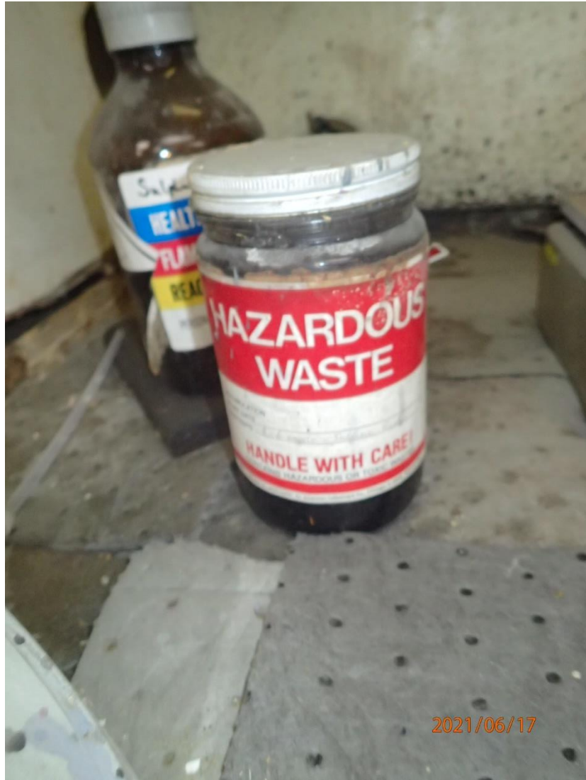
Photo 2: Pint-size glass jar of Sulfuric Acid under a fume hood labeled “Hazardous Waste”, closed, and no indication of hazard
