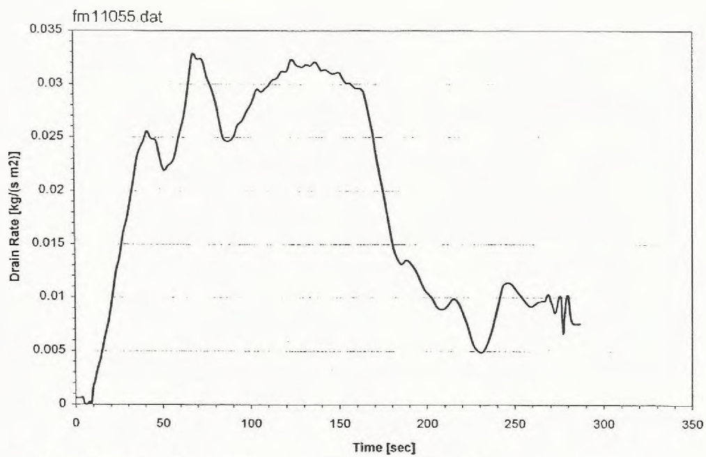
Fig. D59- Drain rate in tests with foam on JP-5 at 50C. Test conditions: expansion ratio= 6.92, irradiance= 50kW/m2, initial foam height= 50mm.
