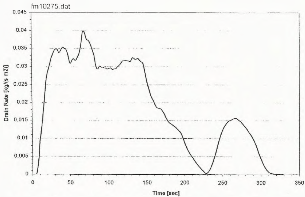
Fig. C163- Drain rate in tests with foam on JP-5 at 20°C. Test conditions: expansion ratio= 5.95, irradiance= 35kW/m², initial foam height= 50mm.
