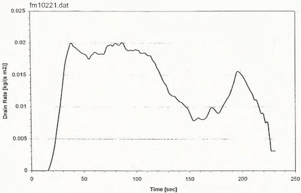
Fig. C283- Drain rate in tests with foam on JP-5 at 20C. Test conditions: expansion ratio= 9.56, irradiance= 50kW/m 2 , initial foam height= 50mm.
