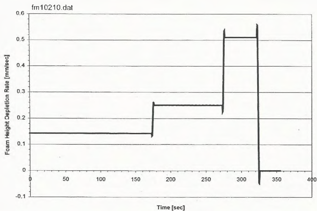
Fig. C272- Foam height depletion rate in tests with foam on JP-5 at 20C. Test conditions: expansion ratio= 8.46, irradiance= 35kW/m2, initial foam height= 75mm.
