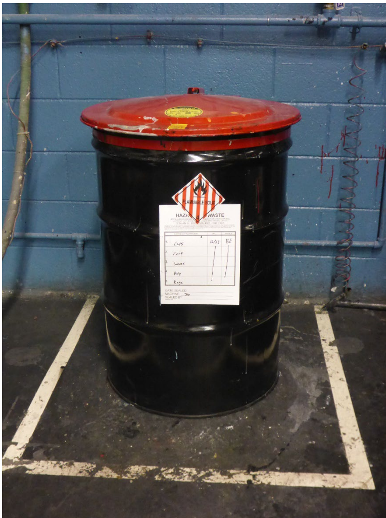
Photo 2: One of three SAAs in the Mix Room for accumulating Stream G hazardous waste solids. This SAA is located in the far corner of the room. The 55-gallon drum in this SAA is labeled hazardous waste solid chips and it is marked with a flammable solids DOT hazard placard. It is not marked to indicate the contents are toxic.
