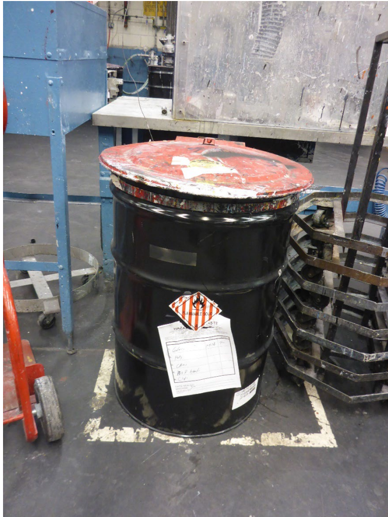
Photo 3: One of three SAAs in the Mix Room for accumulating Stream G hazardous waste solids. This SAA is located in the middle of the room. The 55-gallon drum in this SAA is labeled hazardous waste solids and it is marked with a flammable solids DOT hazard placard. It is not marked to indicate the contents are toxic. The container lid does not make complete contact with the top of the container.
