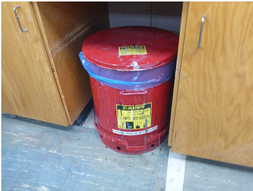
Photo 16: One of two 14-gallon step-to-open flammable cans in the Color Laboratory SAA for accumulating Stream G hazardous waste solids. The container is not labeled hazardous waste, and it is not marked with an indication of the hazards of its contents. In addition, the original “oily rags” and “empty every night” labels are still visible on the container.
