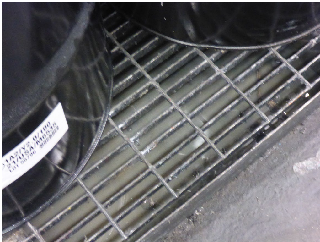
Photo 10: Hazardous waste liquid observed in the portable secondary containment unit beneath six 55-gallon drums of hazardous waste in the middle of the Mix Room. This secondary containment pallet appeared to be a container holding hazardous waste at the time of the inspection, and that container was neither closed nor labeled.
