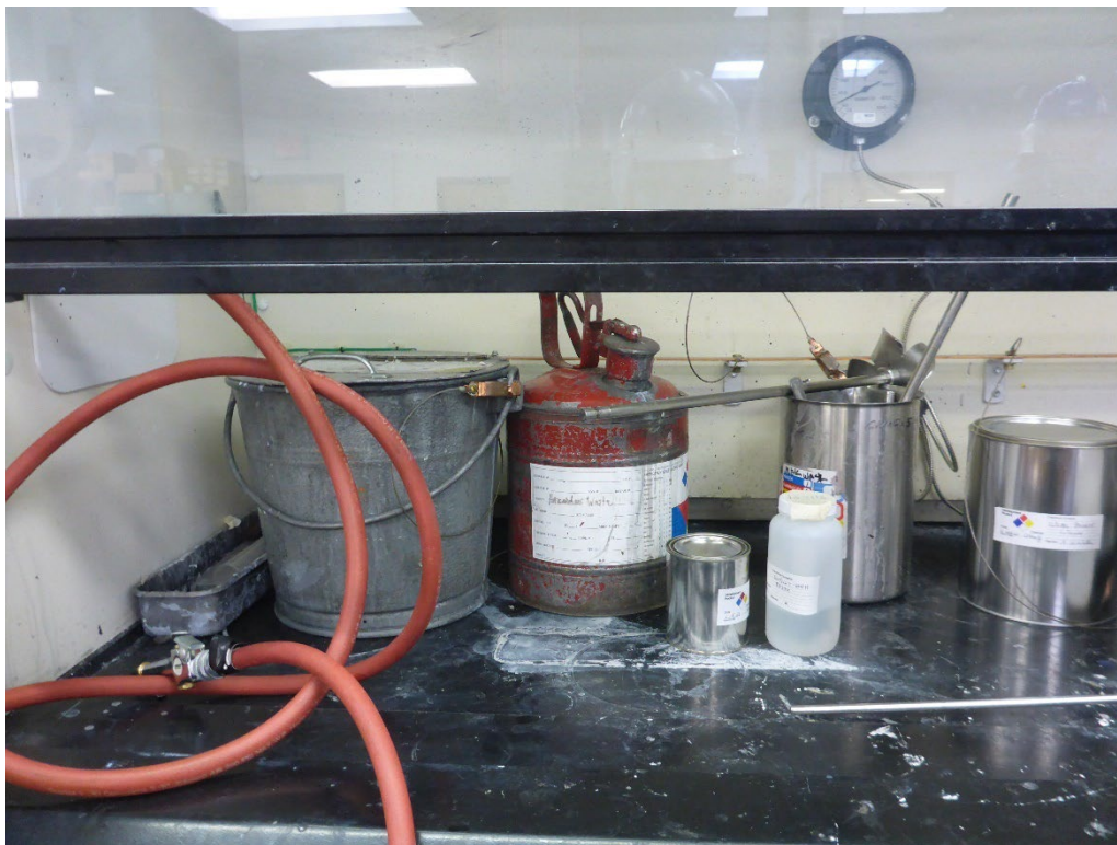
Photo 13: One of red 2-gallon container in the Film Laboratory SAA for accumulating Stream A hazardous waste liquids. The container is labeled hazardous waste, and it is marked with an NFPA fire diamond. However, the numbers marked on the fire diamond had smudged off and were no longer legible.
