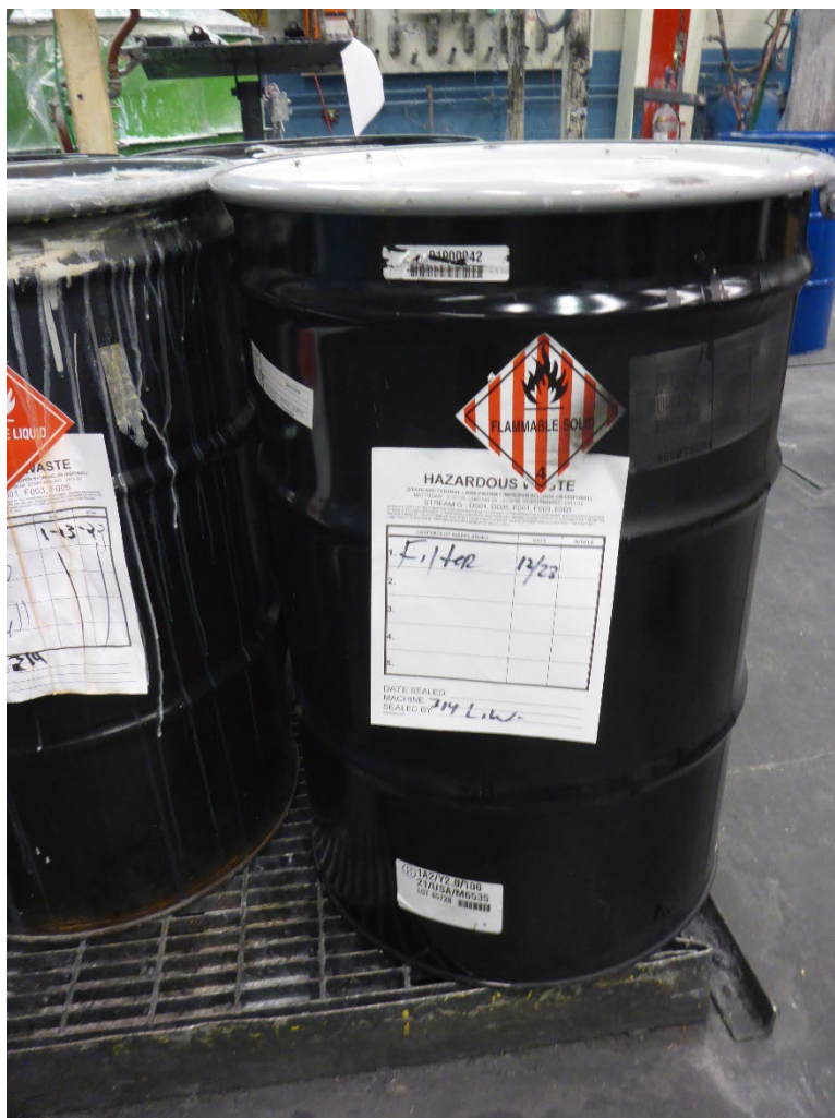
Photo 6: Closer view of two of the ten 55-gallon drums of hazardous waste observed on portable secondary containment pallets in the Mix Room near the Distillation Unit shown in Photo 5. It is not marked to indicate the contents are toxic.
