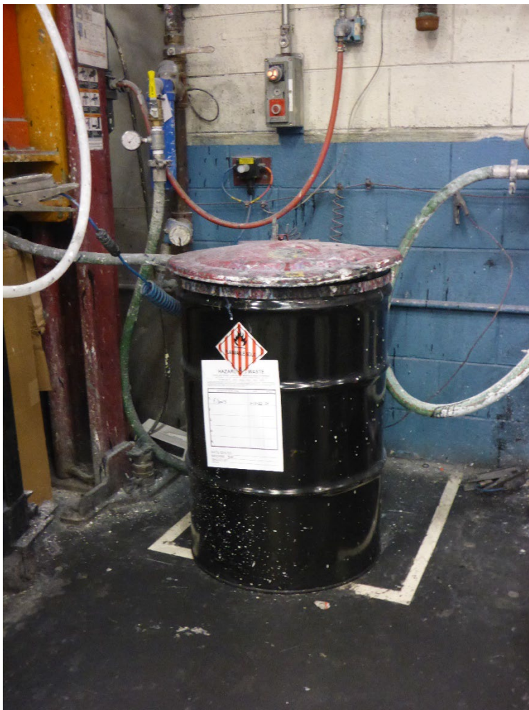
Photo 1: One of three SAAs in the Mix Room for accumulating Stream G hazardous waste solids. This SAA is located next to the CMX-200 Tank Washer. The 55-gallon drum in this SAA is labeled hazardous waste solid filters and it is marked with a flammable solids DOT hazard placard. It is not marked to indicate the contents are toxic.
