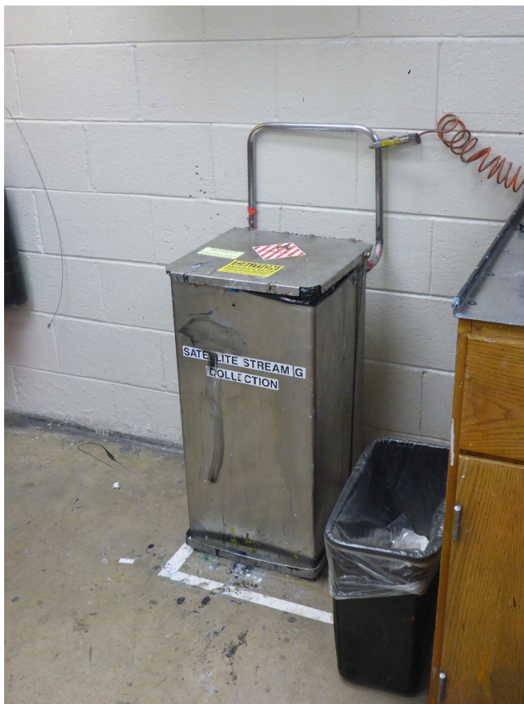
Photo 17: One 30-gallon step-to-open can in the Mix Room Laboratory SAA for accumulating Stream G hazardous waste solids. The container is labeled hazardous waste, and it is marked with a flammable solids DOT hazard placard. It is not marked to indicate the contents are toxic.
