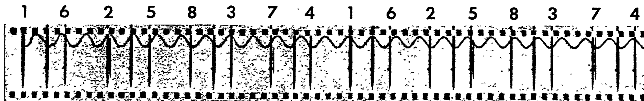
Fig. 2 This cinema film, exposed by the instrument shown diagrammatically above during acceleration of an eight-cylinder car on the road, is a record of the ignition timing of each cylinder. The left edge of the firing mark under each number indicates the instant of ignition. The unnumbered lines are fly-wheel reference marks, 180 degrees apart. The oscillatory curve at the top is a record of the movement of the constant-frequency vibrator. Note that the firing mark for number one cylinder is intentionally made wider by the apparatus in order to identify that cylinder and thus the firing order. Ignition timing of the individual cylinder is read from a curve of angular displacement of the crankshaft versus time, obtained from the flywheel reference points.
