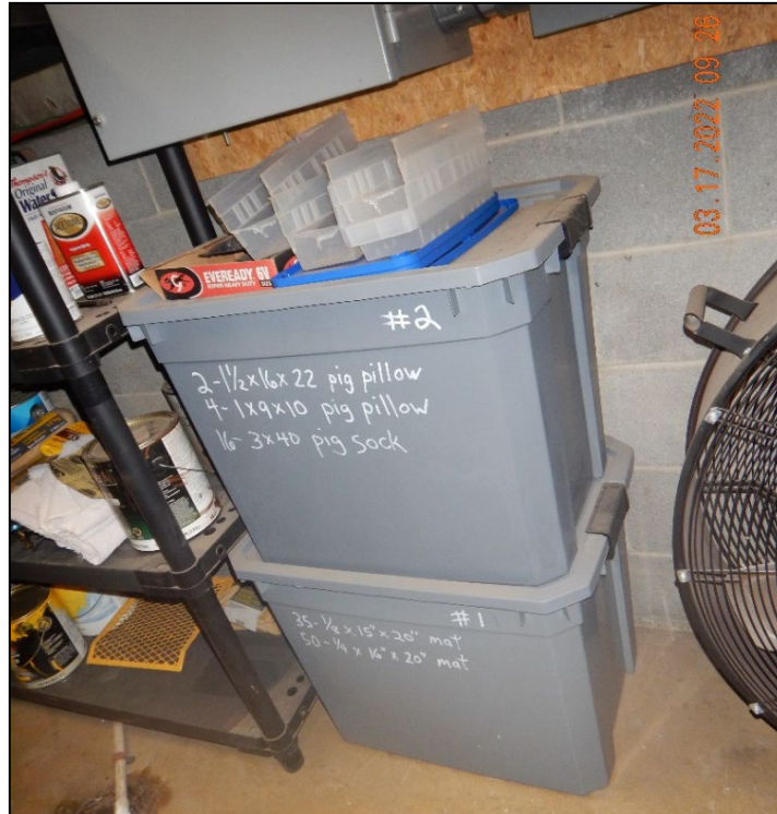
Photograph 9. Township Municipal Building: (DSCN3646.JPG) View of the spill kit located inside the vehicle maintenance garage in the Municipal Building, adjacent to the ASTs.
