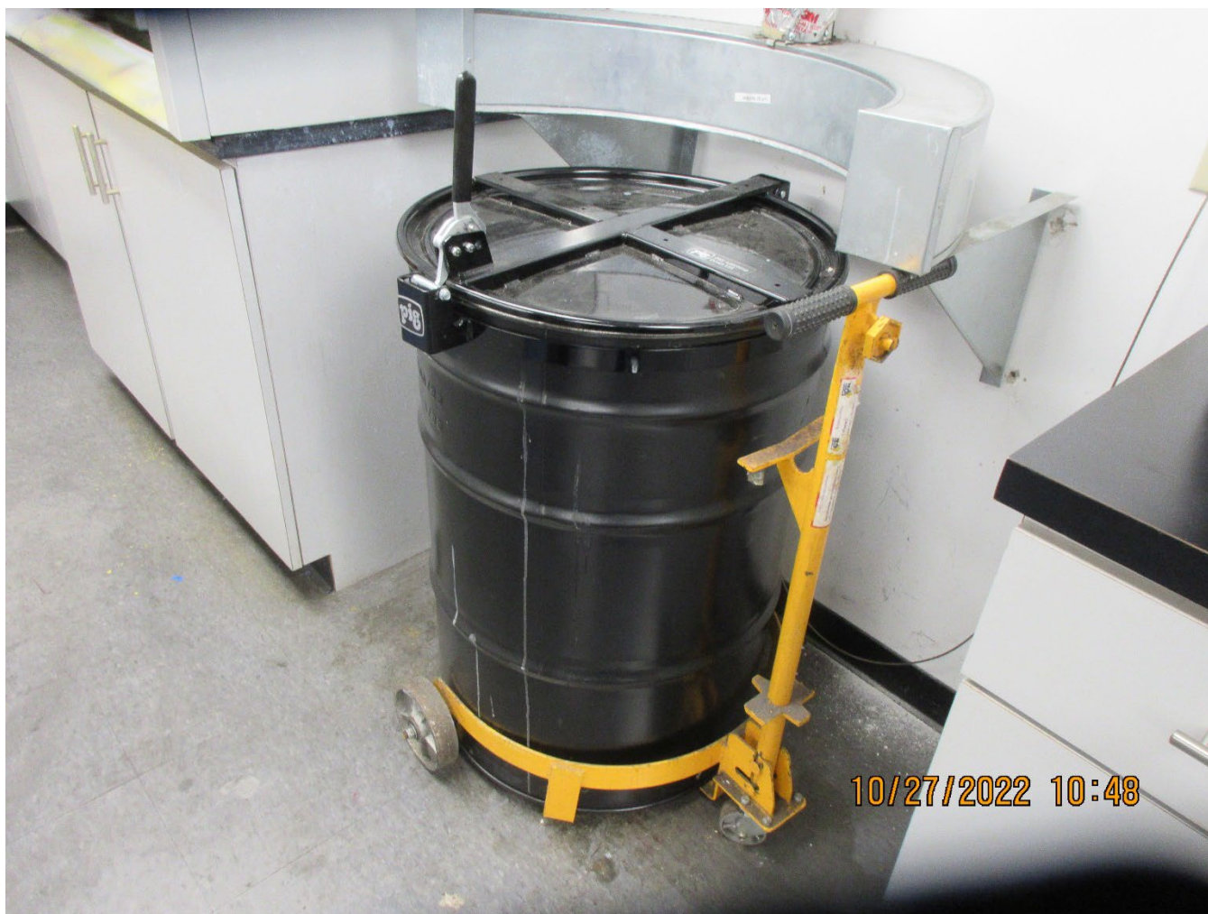
Photo 1 – 55-gallon hazardous waste drum in Quality Control Lab without labels
