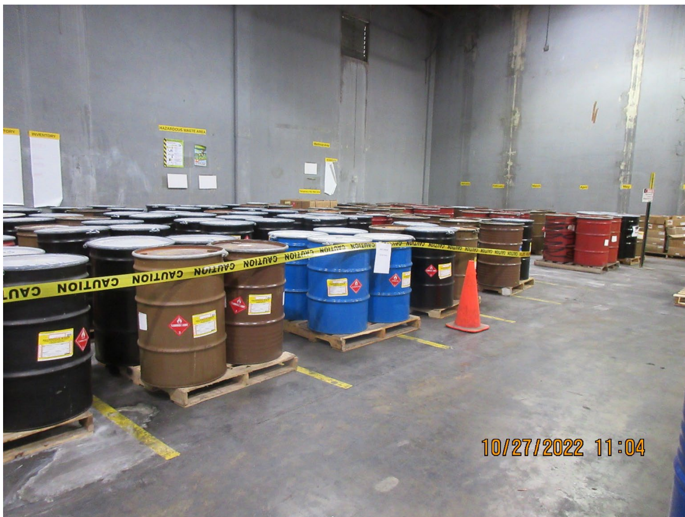
Photo 3 – Drums of Hazardous Waste in Central Accumulation Area
