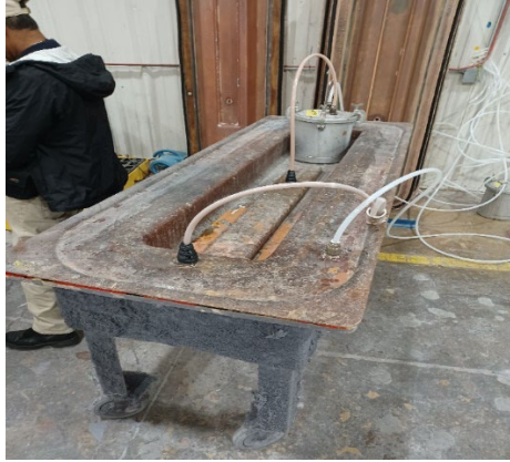
Photo-1 Resin Pumping Station
