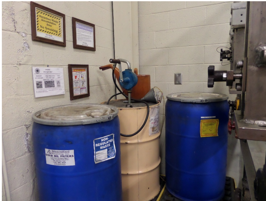
Photograph 13: Propulsion Building – Hazardous waste 55-gallon container and 55-gallon container of used oil contaminated filters in SAA 008 at the Propulsion Building. The hazardous waste container was not marked with an indication of the hazards of its contents.
