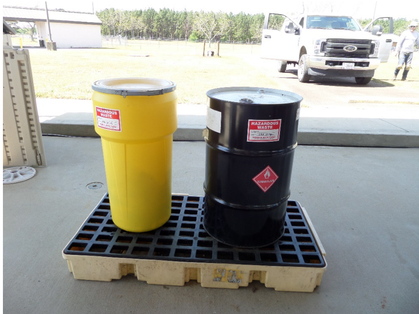
Photograph 12: Hazardous waste containers in the SAA at the loading/distribution station for the petroleum products used at the facility.
