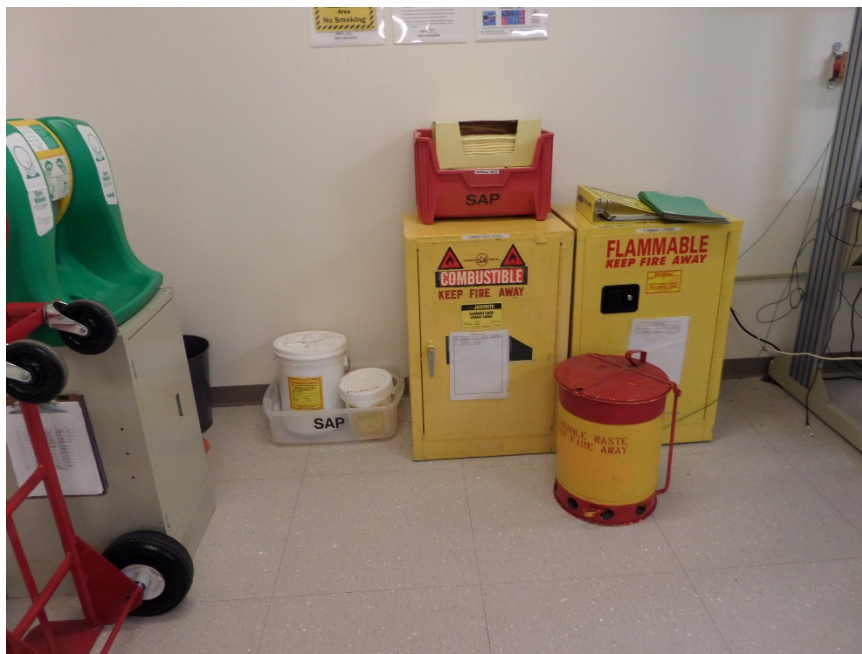
Photograph 14: Avionics Intermediate Section - Hazardous waste in SAA 002. Neither the hazardous waste paint waste container nor the hazardous waste leaded solder flux waste container was marked with an indication of the hazards of its contents.
