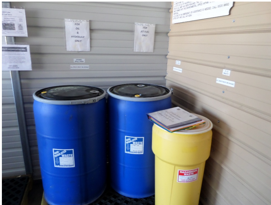
Photograph 10: Containers in the SAA at the Flight Line Maintenance Area. activities of aircrafts fuel systems. The hazardous waste container (14-gallon yellow container) was missing the ring that secures the container’s lid.
