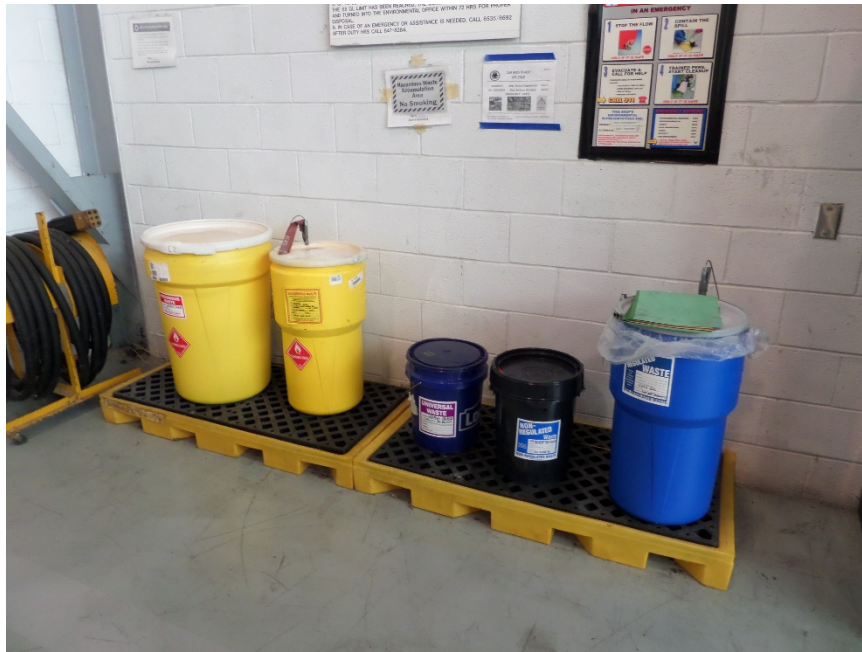
Photograph 9: Containers observed in the SAA at the “Phase” Inspection Area. All containers were properly closed, labeled, and appeared to be in good condition.
