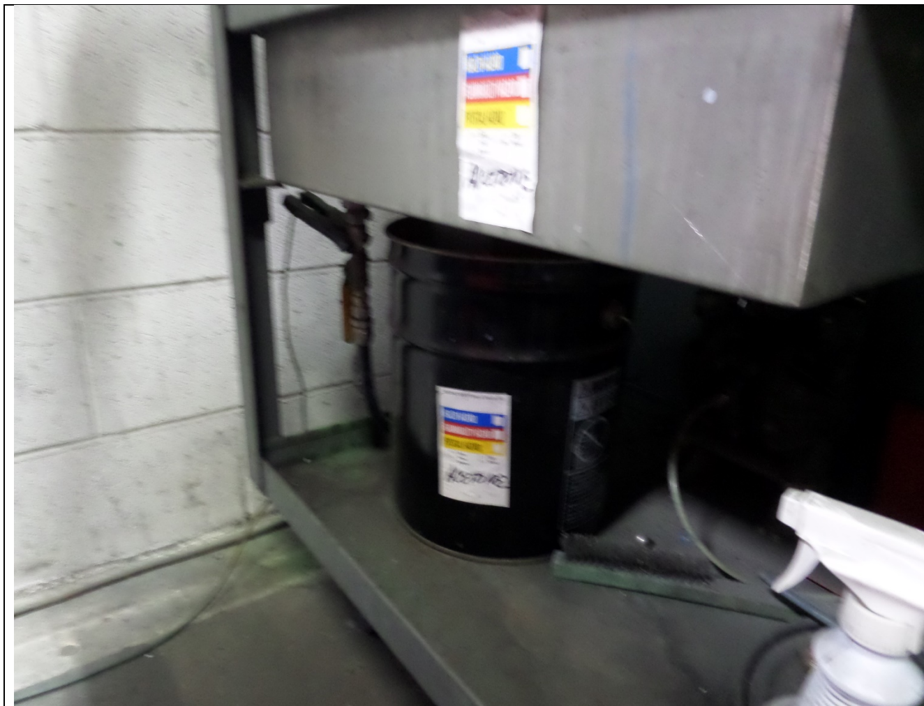
Wilbert. Paint Department. Paint Maintenance. Observed a container not kept closed and was not marked/labeled with the words hazardous waste. Photograph 13 taken at 11:58 a.m.
