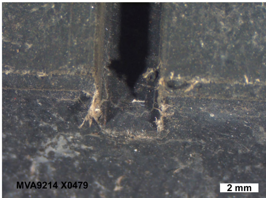
Figure 4. Asbestos fibers are protruding from the surface of Sample X0479A.
