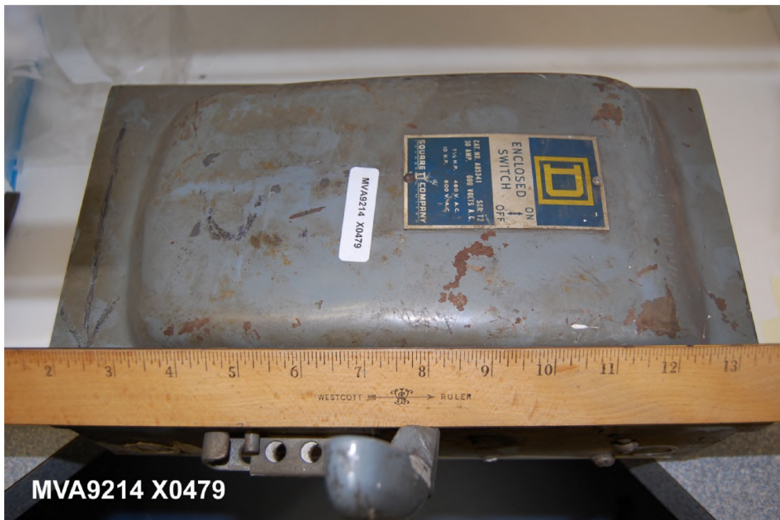
Figure 2. Cover on Sample X0479 (SQUARE D electrical control unit). Label: Enclosed Switch, Cat. No. A85341, SER. T2, 30 AMP, 600 Volts A.C.
