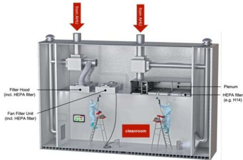
Figure 3.9: Cleanroom ventilation system.
