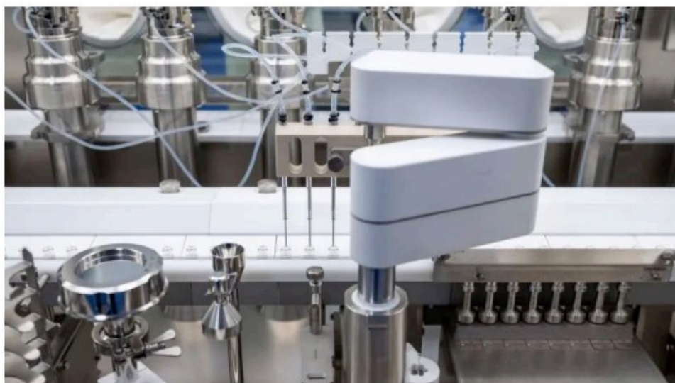
Figure 4.8: Filling line in pharmaceutical production (source: Synthegon)
