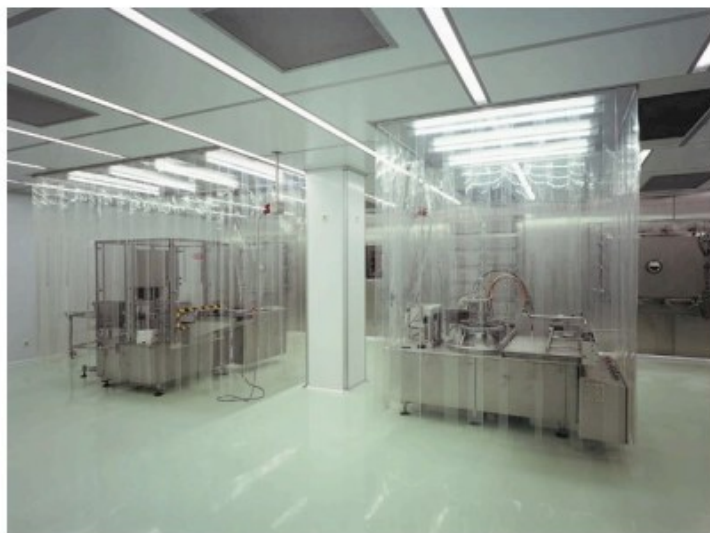
Figure 4.2: Highly clean cleanroom area separated with curtains.
