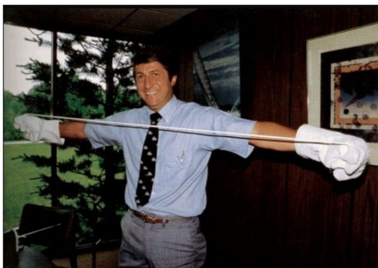
Figure 3.3: Bob Gore stretching (expanding) a PTFE tape [2].
