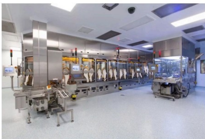
Figure 4.3: Isolator in cleanroom (source: Optima).
