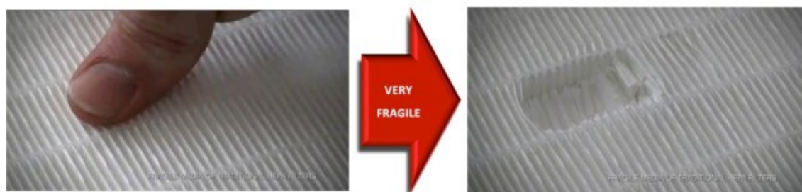
Figure 6.2: Glass fiber media can be easily damaged.
