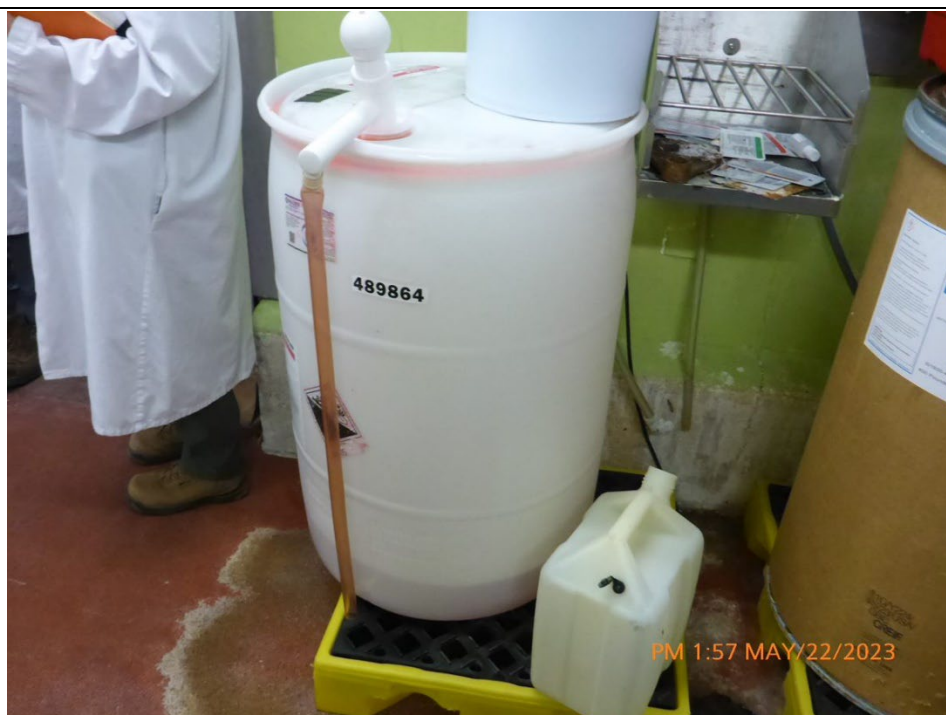
Photograph 5. Improper use of secondary containment for chemical storage at Kunzler.
