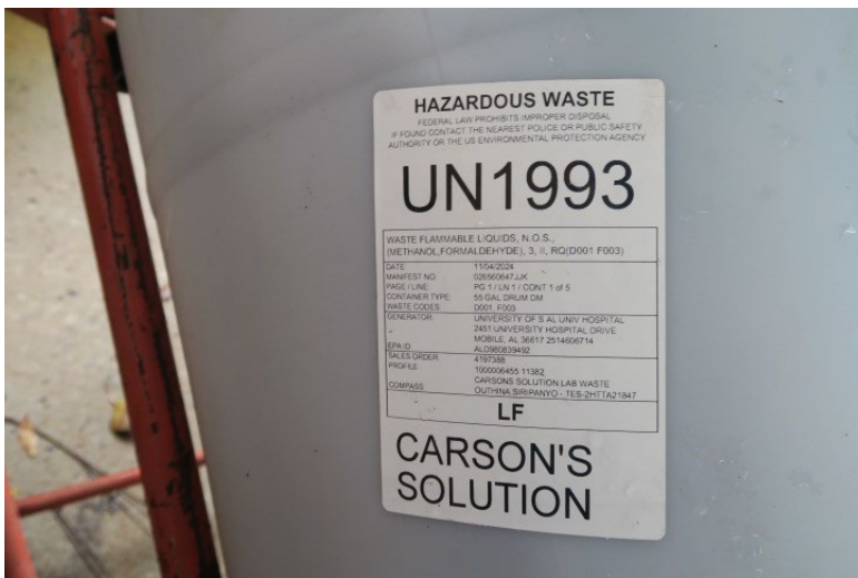
Photo 2: Hazardous waste label on the 30-gallon drum of hazardous waste labeled Carson's Solution in the TSD Building outdoor staging area
