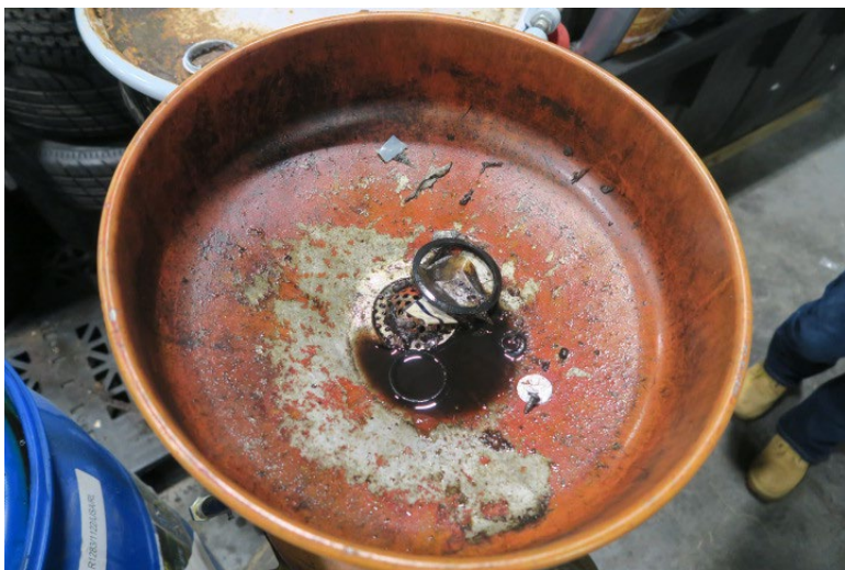
Photo 26: Oil residue in the funnel of the container used to transfer used oil. Located in the Grounds/Transportation Maintenance Area.
