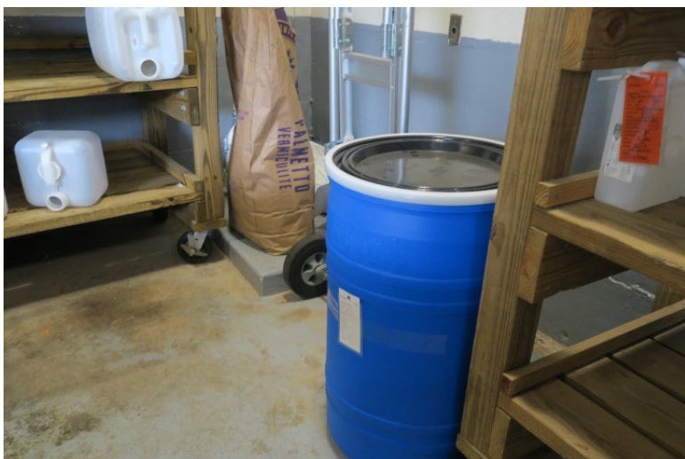
Photo 16: one 30-gallon drum containing lead vests, that was labeled with waste code D008, an accumulation start date, and a hazardous waste label. The container did not have an indication of hazard label. Located next to the wooden shelf for toxic waste (reference photo 10).
