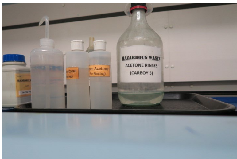
Photo 21: Hazardous waste containers in the fume hood of a chemistry lab in the Science laboratory building SAA. Containers were labeled with the words hazardous waste but did not contain indications of hazard.
