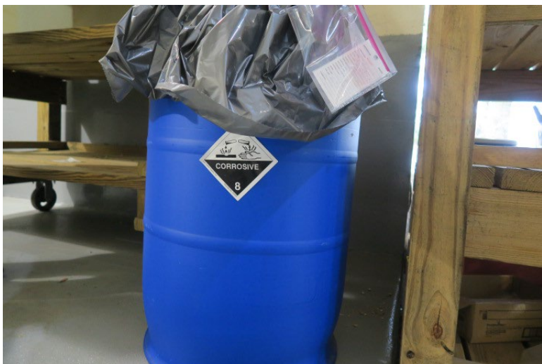
Photo 15: One 30-gallon hazardous waste drum labeled with the words "hazardous waste," corrosive hazard indicator, waste codes, and accumulation start date. Located next to the wooden shelf for toxic waste (reference Photo 14).
