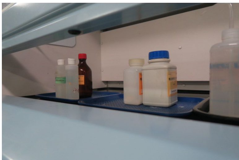
Photo 20: Hazardous waste containers in the fume hood of a chemistry lab in the Science laboratory building SAA. Containers were labeled with the words hazardous waste but did not contain indications of hazard.
