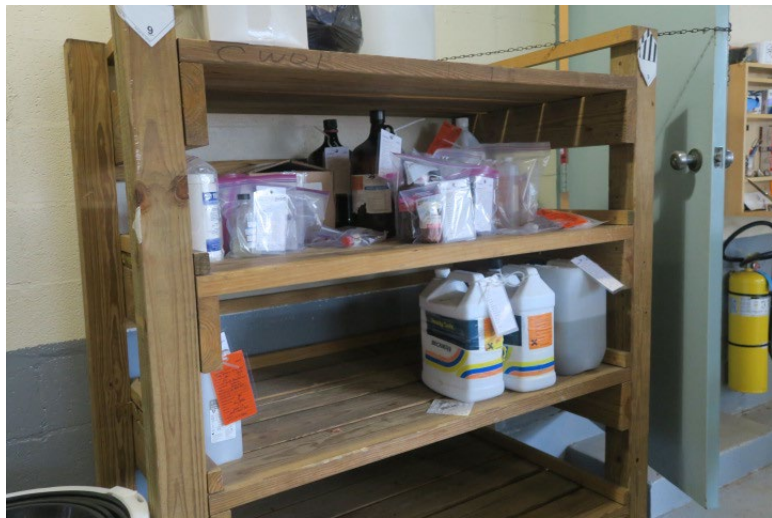
Photo 10: Waste containers on the wooden shelves at the incoming waste processing area in the TSD Building, shelf labeled with Toxic hazard indicator for miscellaneous toxic waste storage.
