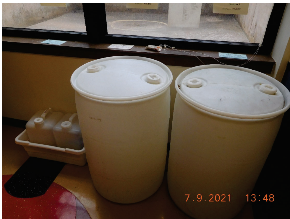
Photo 5: SAA in Ekeley Sciences room M1B10 with two 55-gallon containers and two 5-gallon containers of solvent waste. Containers are not labeled as hazardous waste; labels are on the signs on the windowsill. (DSCN1415.JPG)
