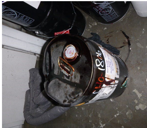
Photograph 20: Pooling of product on ground and container - P1030627.JPG
