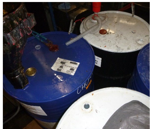
Photograph 28: Open drums in Aerosol SAA - P1030635.JPG
