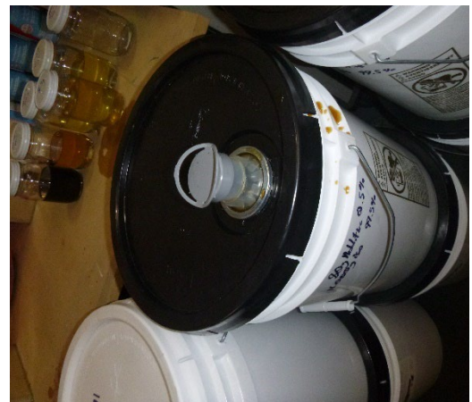
Photograph 6: Pooling on product bucket - P1030614.JPG
