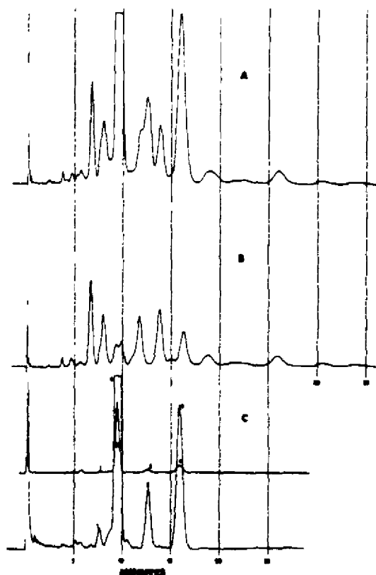
FIGURE 15. Gas chromatograms of sample from salmon from Lake Michigan. A is before separation of pesticides from PCB, B is PCB after separation and C is DDT pesticides.
