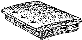
Type ventilate "E" used for medium duty slip applications.
